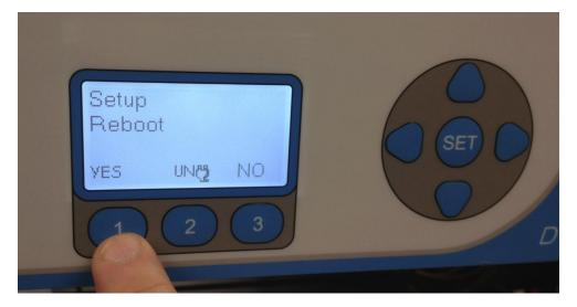
For a full shutdown, the power must be pulled from the XDS satellite receiver, wait 15 seconds, then apply the power (plug in to AC).
