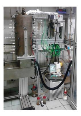
Semi-continuous fluidized bed H: 60 ੴA? ☞ = 6 cm Raw biomass: 80 g Particle size: 2-3 mm
