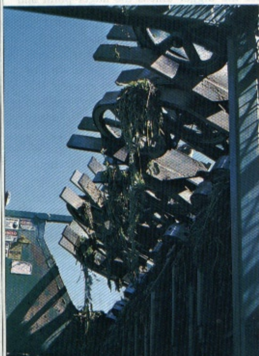
Pulleys at the top of the harvester bring the carrots up from the surface, and rotating blades cut off the carrot
