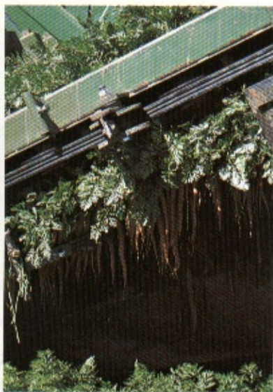
Carrots travel up a series of belts to the top of the harvester where the tops are cut off and fall onto a conveyor belt that drops the carrot into the truck.
