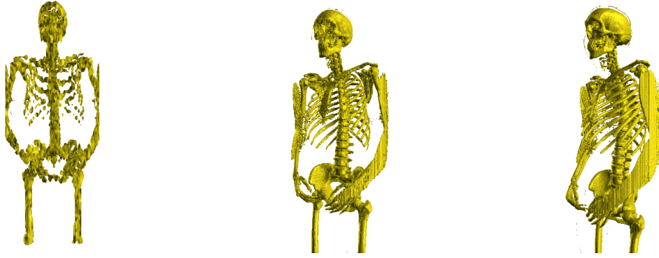
Figure 4: An isosurface for the Male MRI data (isovalue = 1200) is progressively extracted and rendered at different resolutions and from various viewpoints. The leftmost isosurface has 24, 084 triangles; the center isosurface has 651, 234 triangles, and the rightmost isosurface has 6, 442, 810 triangles.
