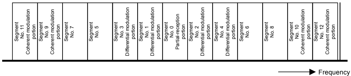
Fig. 3-30: OFDM-Segment Numbers on the Transmission Spectrum and Example of Usage (13-segment Type)
