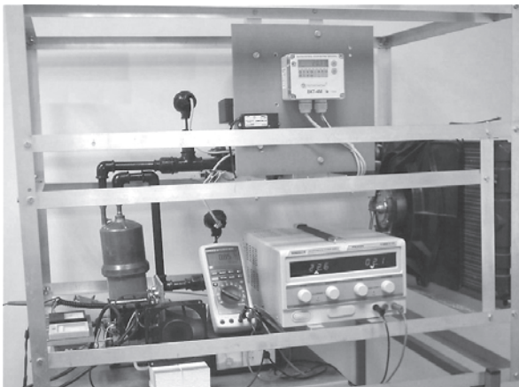
Fig. 4. The experimental device for hydrogen recombination research
