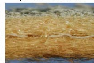
Dust stays more on the spunlaced filter surface
