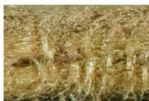
Dust penetrates more into the core of a needle felt
