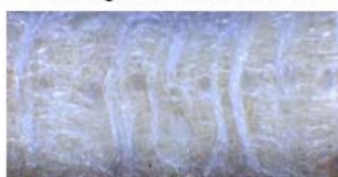
Dust penetrates more into the core of a needle felt
