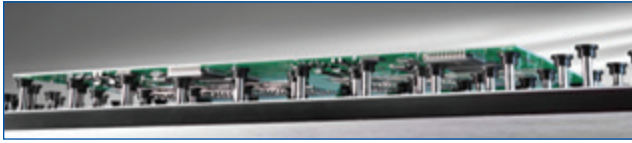
FIGURE 4. Flexible support system. Note how the system conforms to the PCB bottom's profile.
