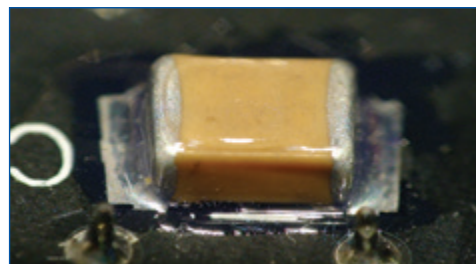
FIGURE 1. A capacitor manually coated with conformal coating under normal lighting.
