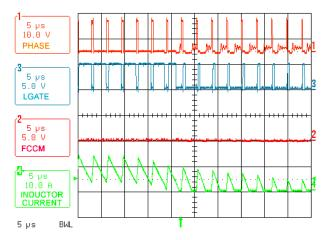
FIGURE 3. LOAD TRANSIENT (30 - 0A, 3-PHASE)
