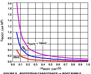
FIGURE 8. BOOTSTRAP CAPACITANCE vs BOOT RIPPLE VOLTAGE
