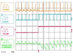
FIGURE 4. DCM TO CCM TRANSITION AT NO LOAD
