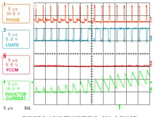
FIGURE 2. LOAD TRANSIENT (0 - 30A, 3-PHASE)
