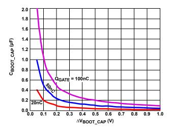
FIGURE 7. BOOTSTRAP CAPACITANCE vs BOOT RIPPLE VOLTAGE
