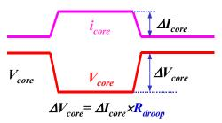
FIGURE 10. DESIRED LOAD TRANSIENT RESPONSE WAVEFORMS
