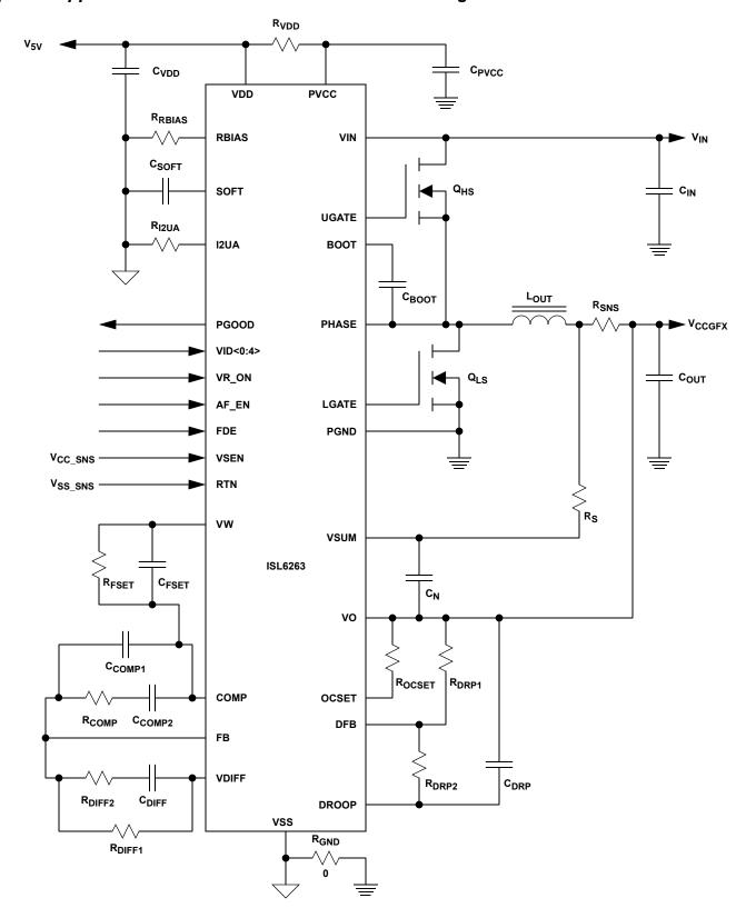
FIGURE 3. ISL6263 GPU RENDER-CORE VOLTAGE REGULATOR SOLUTION WITH RESISTIVE CURRENT SENSING
