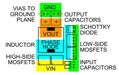
FIGURE 13. TYPICAL POWER COMPONENT PLACEMENT
