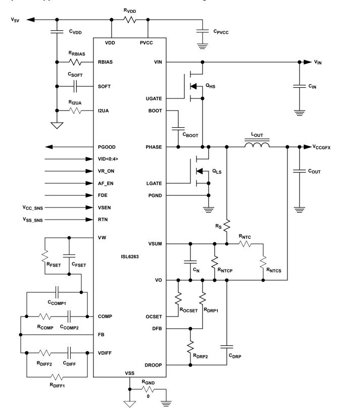
FIGURE 2. ISL6263 GPU RENDER-CORE VOLTAGE REGULATOR SOLUTION WITH DCR CURRENT SENSING
