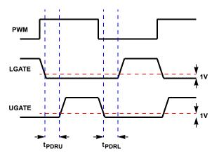
FIGURE 6. GATE DRIVER TIMING DIAGRAM
