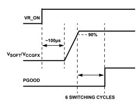
FIGURE 4. ISL6263 START-UP TIMING
