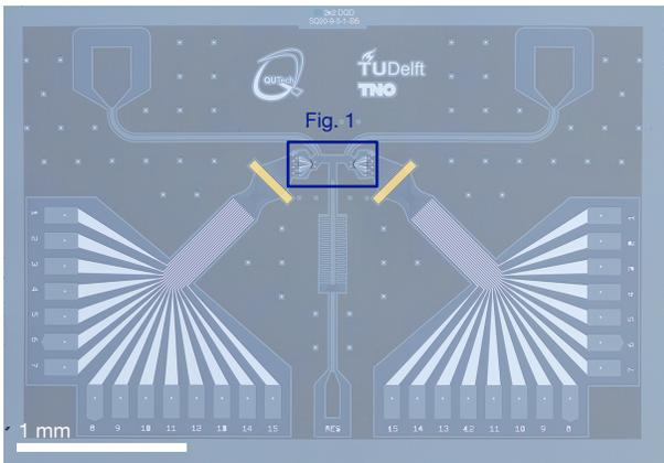
Figure 5. Composite optical image of the device chip without wire bonds.
