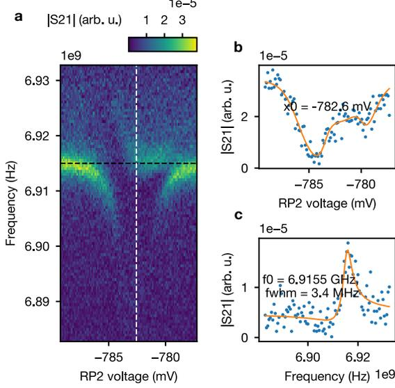
Figure 7. Fitting of zero charge detuning. **(a)** Example of a single frame of data used in a vacuum Rabi splitting reconstruction. **(b)** Cut along the black line from panel (a) corresponding to the bare resonator frequency to extract the zero-detuning gate voltage  $x_0$ . An empiric fitting function is used to find the center of the signal dip due to the dispersive shifts. **(c)** Cut along the fitted zero-detuning value  $x_0$  (white line) and fit to a single Fano resonance.
