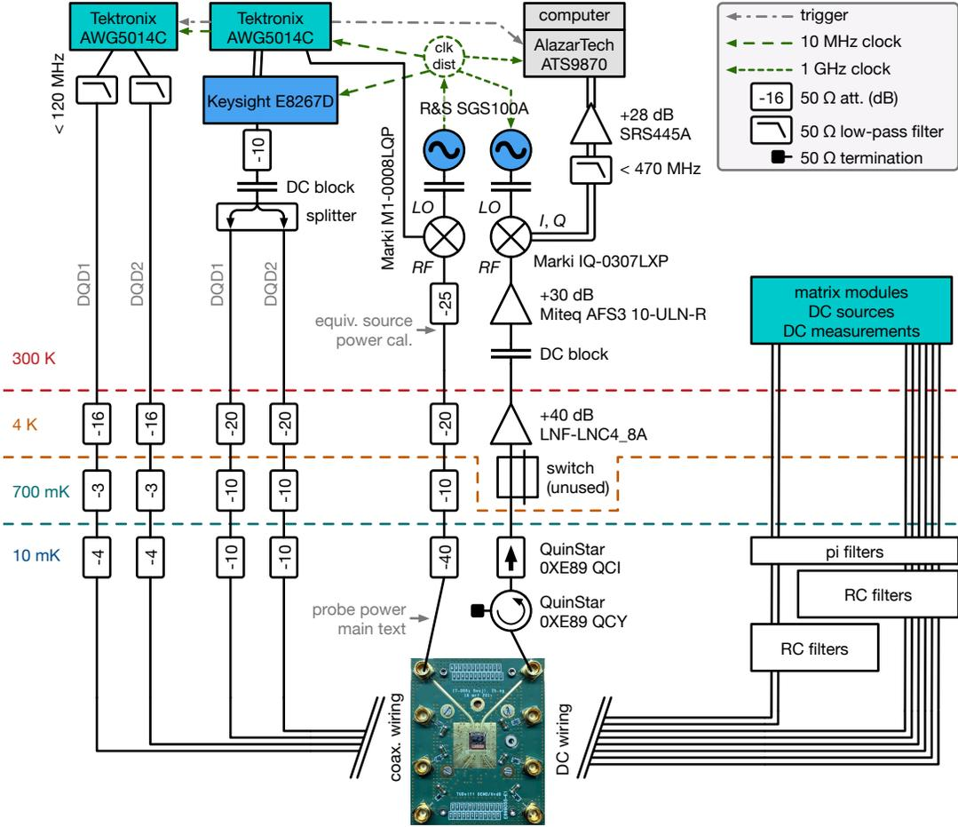
Figure 6. Schematic of the measurement setup.
