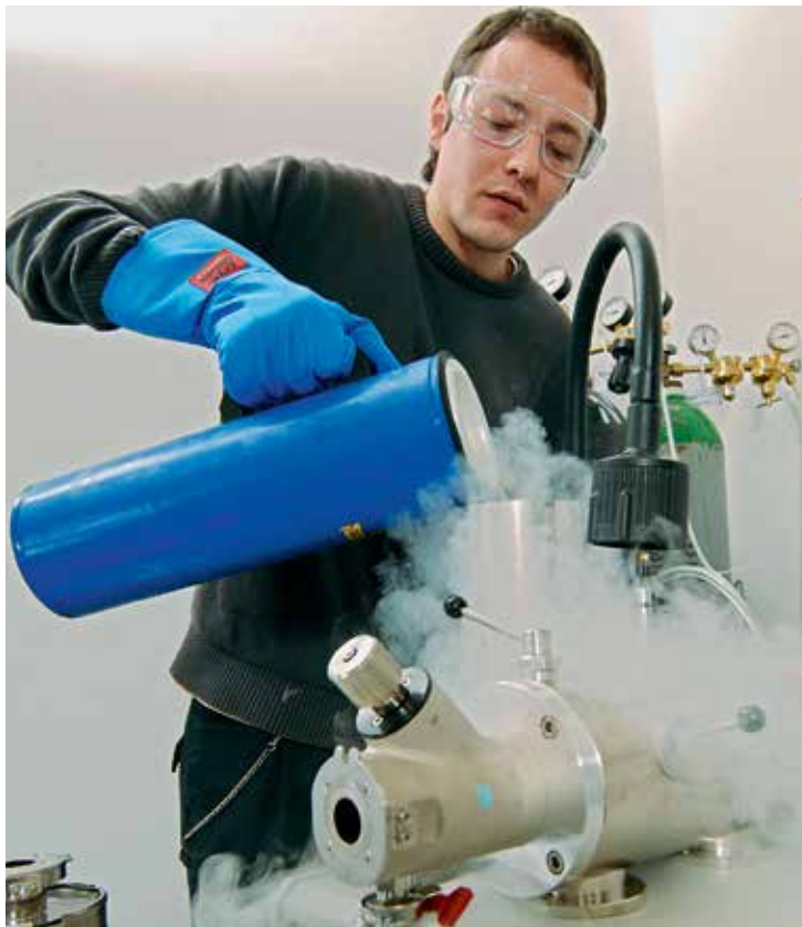
PhD student Oliver Hagedorn freezing samples for examination under a field emission scanning electron microscope (FE-SEM). Right: SEM images of aster pollen (1), glands on a hop leaf (2) top view of highly magnified human hair (3).
