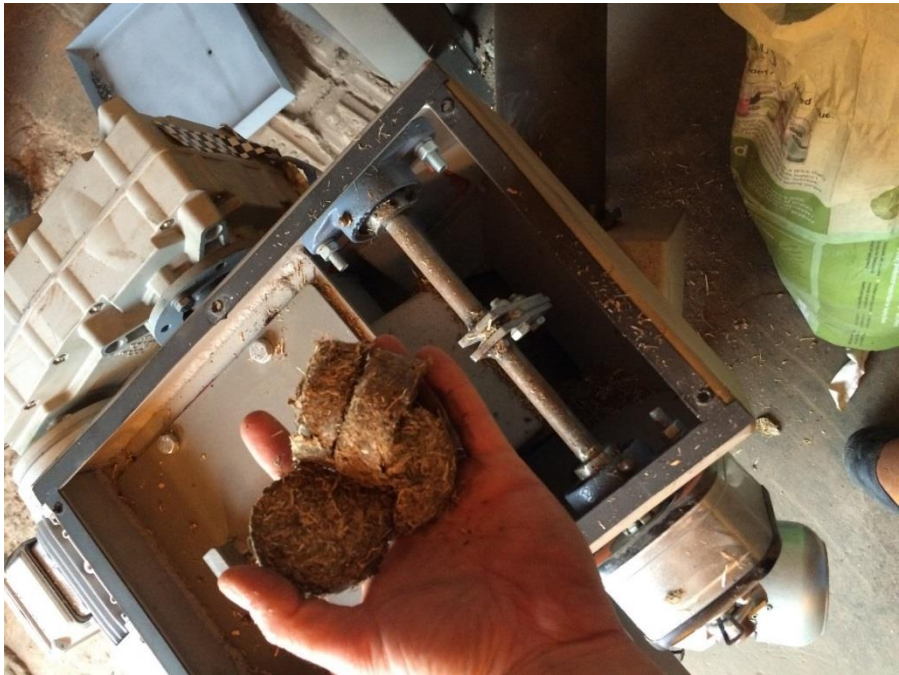
Figure 12 - Ag biomass pucks made from residue from an idle field used for demonstration burns at VFFC.
