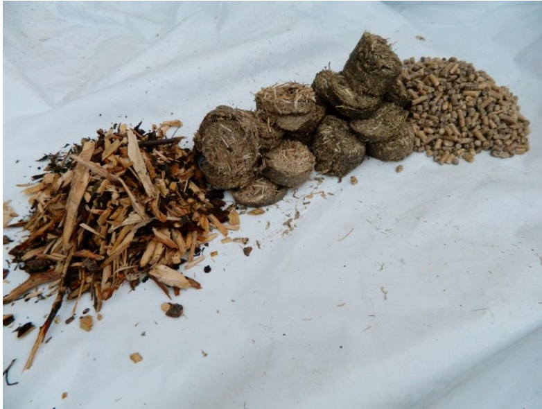
Figure 1 - An assortment of the fuels that the boiler can burn. Left to Right: wood chips, grass biomass fuel pucks, and wood pellets.
