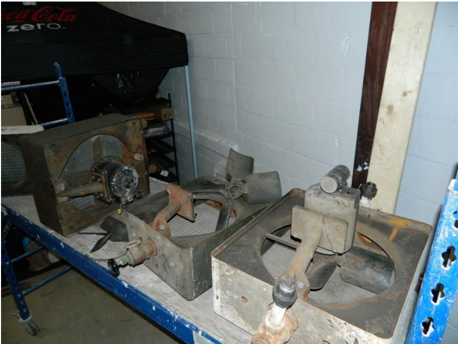
Figure 14 - Several of the salvaged unit heaters prior to pressure testing and electric motor testing.
