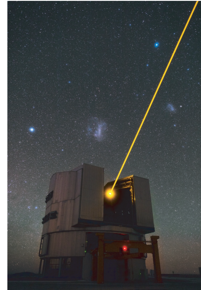
FIGURE 75 The most expensive laser pointer: a yellow 10 W laser that is frequency-stabilized at the wavelength of sodium lamps allows astronomers to improve the image quality of terrestrial telescopes. By exciting sodium atoms found at a height of 80 to 90 km, the laser provides an artificial guide star that is used to compensate for atmospheric turbulence, using the adaptive optics built into the telescope. (© ESO/Babak Tafreshi).
