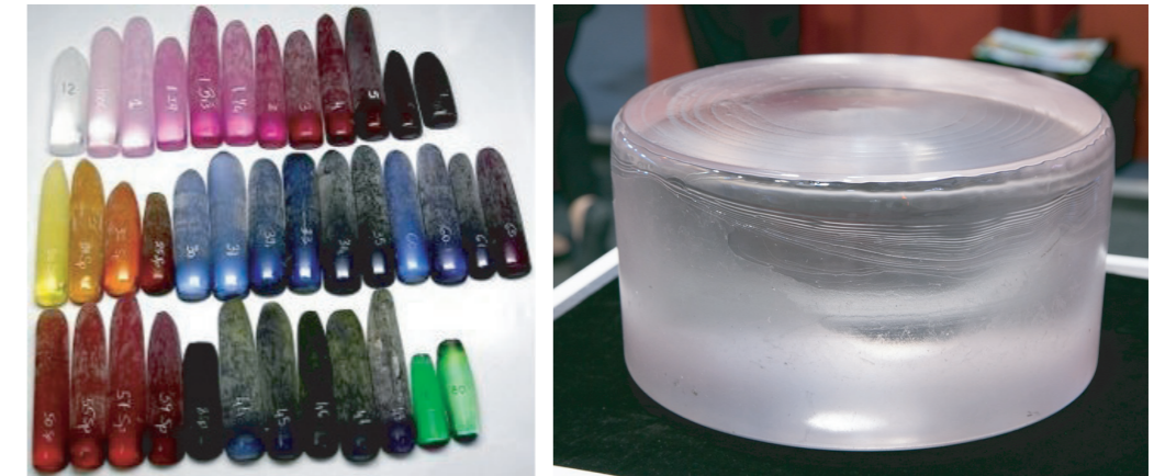
FIGURE 35 Left: raw crystals, or boules, of synthetic corundum, picture size c. 50 cm. Right: a modern, 115 kg corundum single crystal, size c. 50 cm (© Morion Company, GT Advanced).
