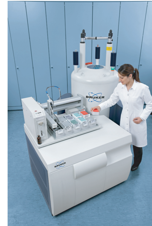
FIGURE 113 A machine to test fruit quality with the help of nuclear magnetic resonance (© Bruker).
