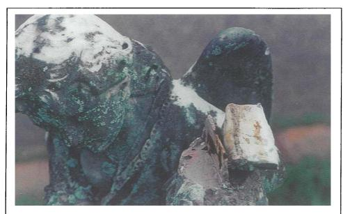
Figure 21. Broken cross (Lot I). Metal wedge will need to be removed before any repairs can be done.
