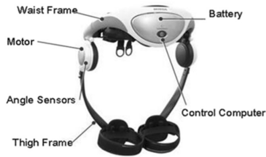
Figure 3: Honda Stride Management Assist (SMA) Device [1].
