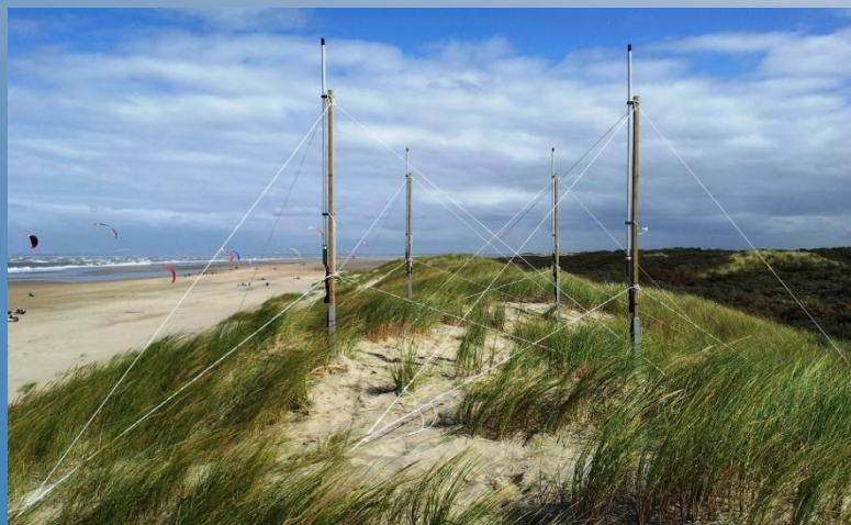
WERA antenna array in the dunes of Ouddorp
