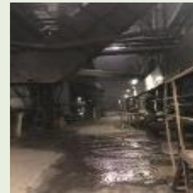
3. Low illumination, water and oil spillage, rusting
