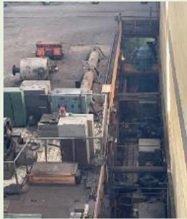
1. Coal dust accumulation was observed in the maintenance bay area
