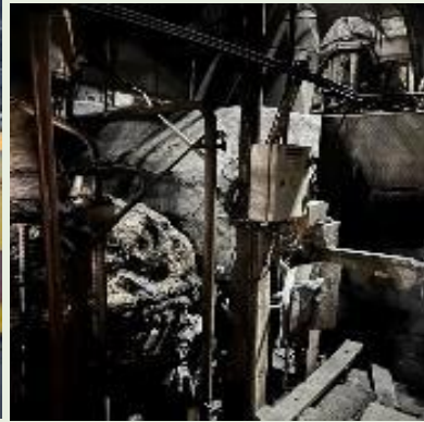
1. High amount of coal dust deposit and debris accumulation seen
