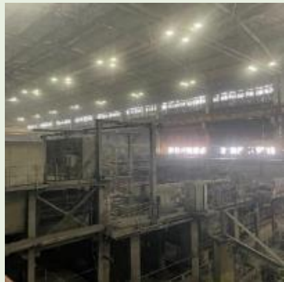
1. Coal dust deposit accumulation and suspension in the atmosphere
