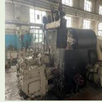
3. Oil stain & deposits and lacks safety system 2
