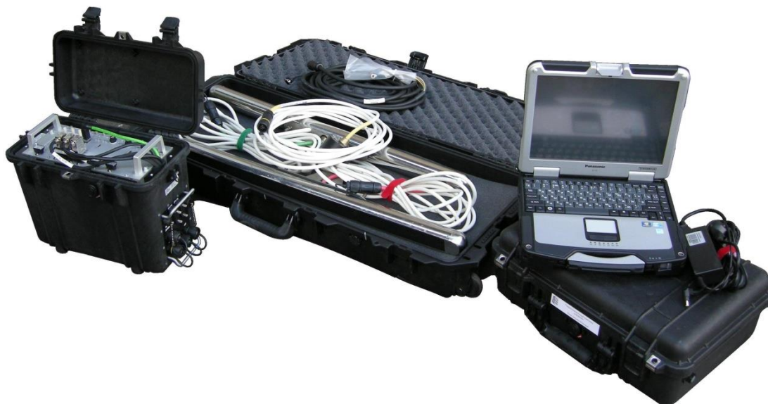
Fig. 2. Mobile side scan sonar complex “Neman GBOE” (general view).
