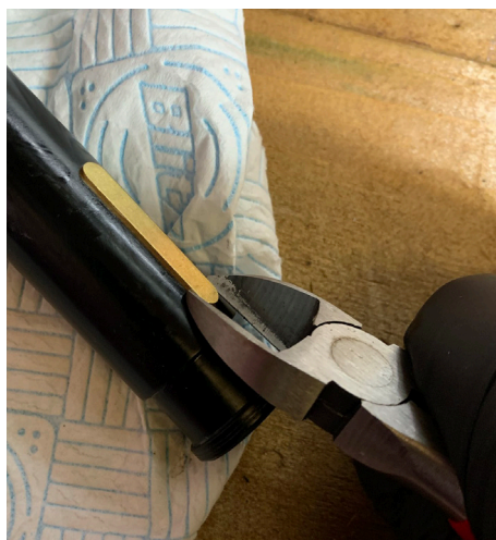
17. Carefully remove the brass keys using side cut pliers to grip them.
