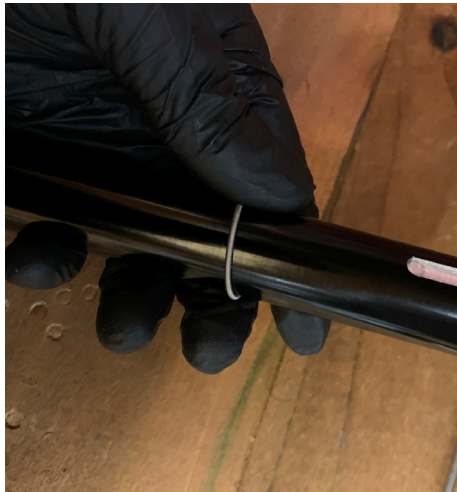
25. Fit metal retaining ring onto the stanchion.
