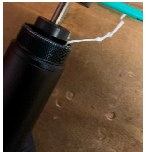
6. Undo and remove bolt on actuator using 2mm hex key then remove actuator from the bottom of the cartridge.
