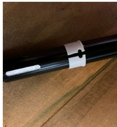
29. Refit top bushing. Note: orientation of this to ensure it is fitted the correct way round.
