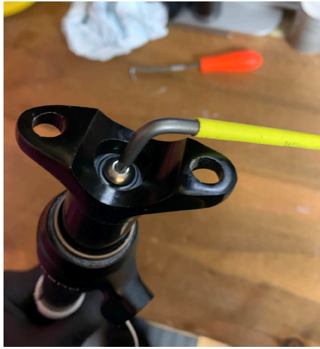
40. Loosely refit bolt to hold cartridge in place using 3mm hex key.
