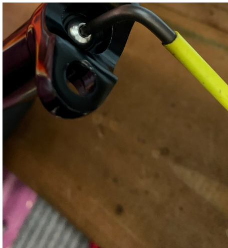
8. Undo bolt on the top of the stanchion using 3mm hex key which is holding the cartridge in place. Note: you may also need to hold the cartridge with your hand.
