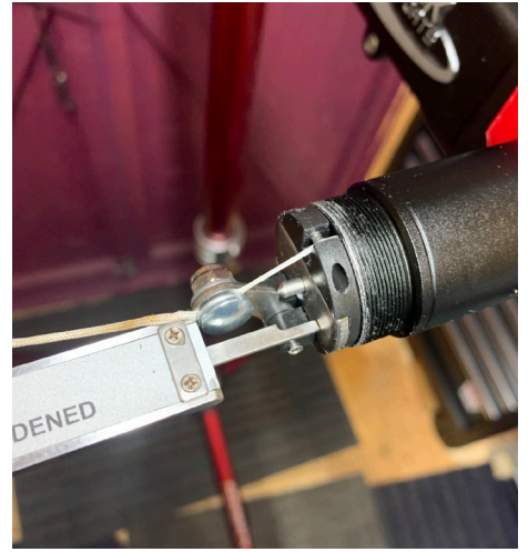
52. Using your Vernier calipers measure the height of the actuator and adjust string so that it is between 20.5mm and 21.5mm then tighten bolt to 4Nm Note: as you tighten be sure not to push on the pin as the seatpost will extend.
