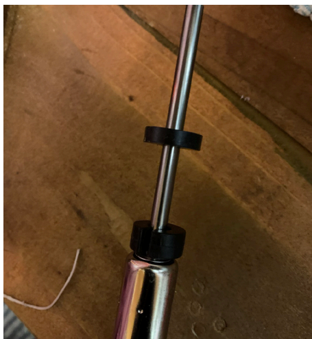
37. Refit bump stop and washer onto the bottom of the cartridge.
