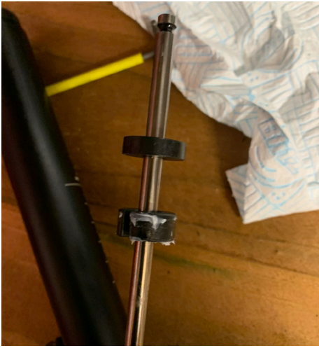
10. Remove bump stop and washer from bottom of cartridge.
