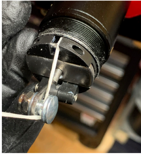
51. Feed string through hole in bolt and washer then push through actuator, add the other washer and loosely tighten nut.
