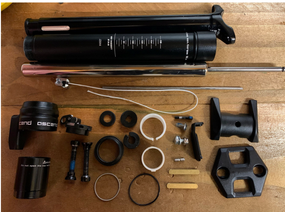
22. Remove the metal retaining ring from the stanchion.
