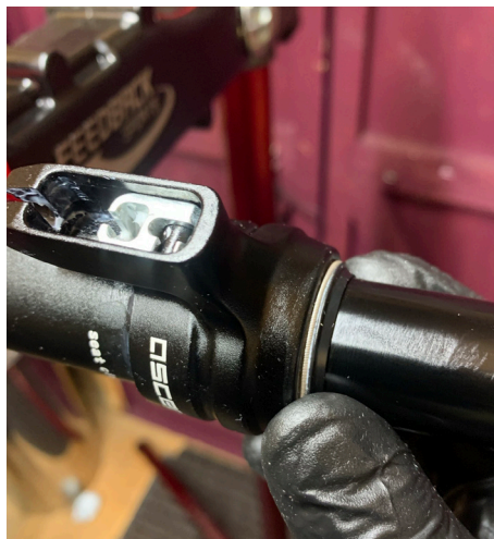
54. Refit metal retaining ring on the collar seal.
