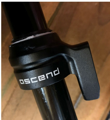
28. Slide collar onto stanchion ensuring seal does not get folded or damaged.
