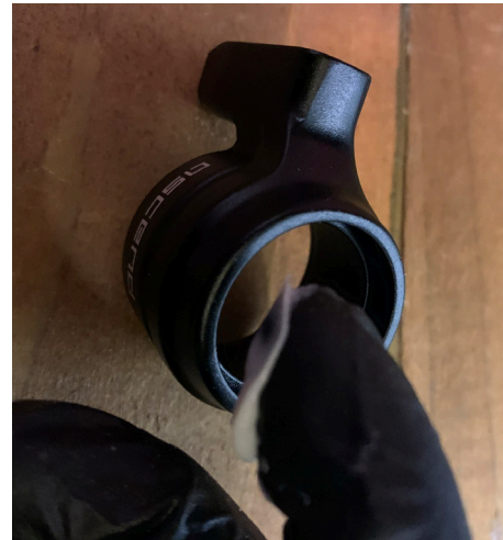
26. Grease inside of collar.
