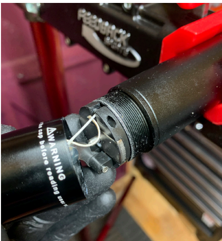
53. Neatly locate any excess string then replace bottom cap and tighten to 5Nm.
