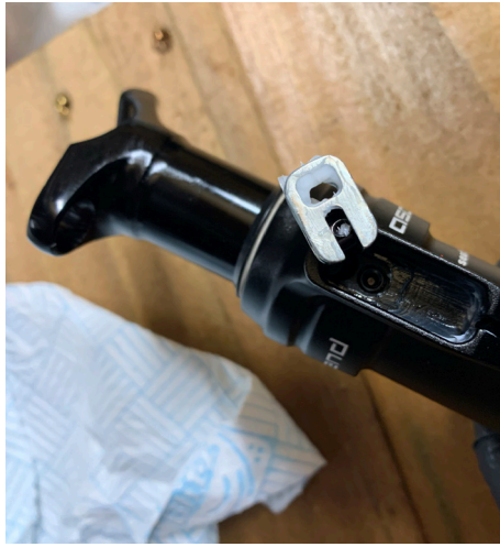
11. Pull the metal cable guide and string out from the post.
