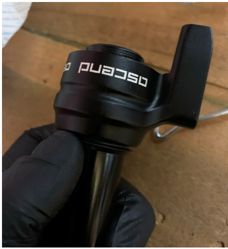
20. Remove the collar from the stanchion.
