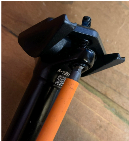
2. Remove seat clamp bolts.
