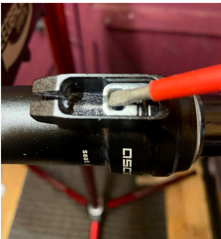
56. Using a flat head screwdriver, push down on the silver cable guide to extend post, push the silver cable guide again and compress post to check function.
