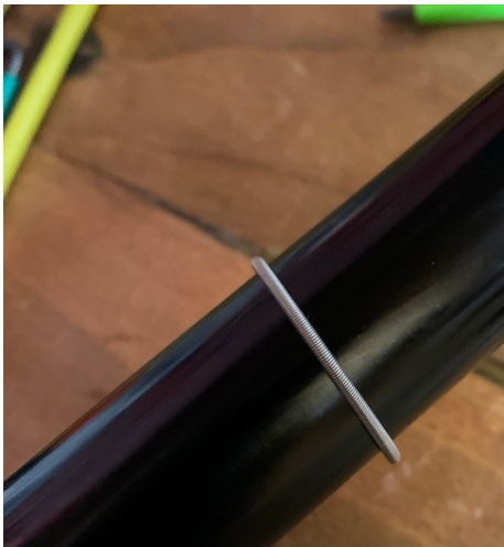
22. Remove the metal retaining ring from the stanchion.
