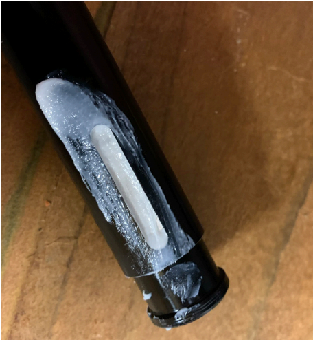
30. Grease seats for the brass keys.
