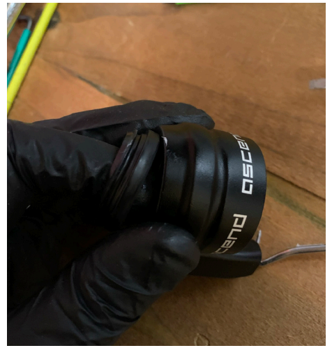
21. Remove the seal from the collar.
