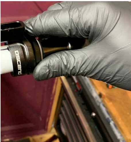
13. Carefully pull the collar to slide it up the stanchion and remove it from the lower part of the post.
