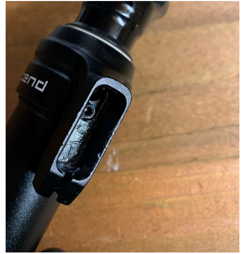
12. Loosen bolt on the collar using 2.5mm hex key.
