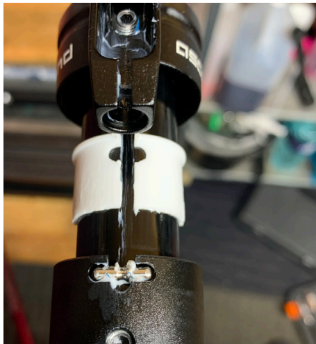
14. Note the position of the bushing and actuator – remove the stanchion from the lower part of the post by carefully pulling it out.
