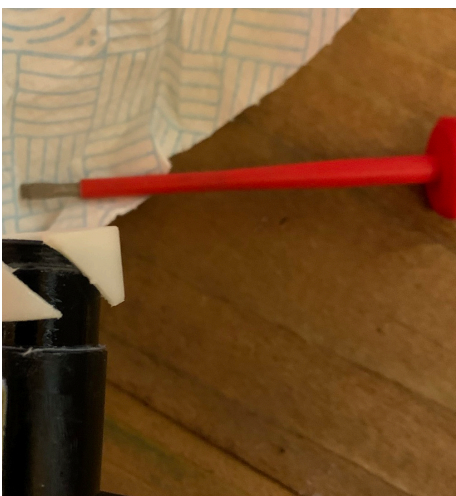
16. Remove the lower bushing.
