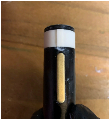
34. Rotate bushing so that the ridge is in line with one of the brass keys.
