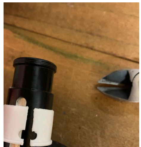
18. Remove the upper bushing.
