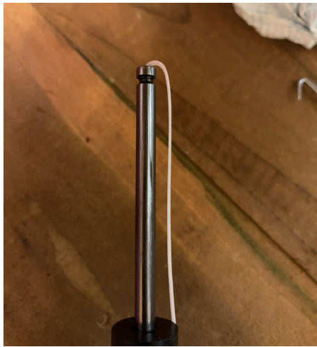
42. Feed excess string inside the cartridge, you can secure with an elastic band to added security.
