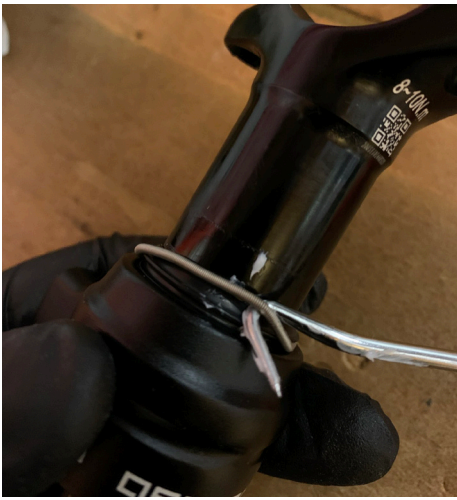
19. Slide the metal retaining ring off the seal.
