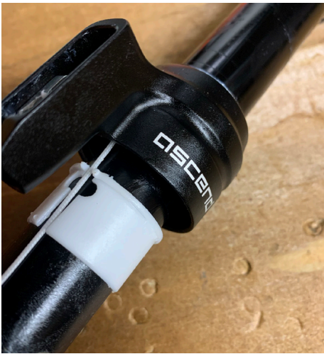
41. Rotate the collar, string and bushing so everything is lined up. The string should go through the slot in the bushing.
