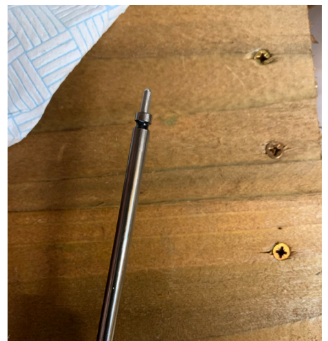
38. Double check your cartridge has been compressed halfway. If it is still at full extension insert the pin and push down on the end to compress.
