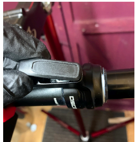
57. Replace cable cover.
