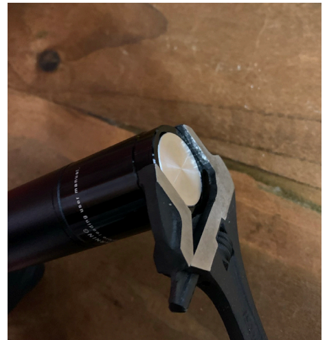
3. Remove cap on bottom of post using 28mm spanner.
