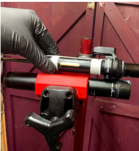
43. You are now ready to slide the stanchion into the lower part of the post. Visually line up the rear of the stanchion (the side with the etching on the rear) with the rear of the lower part of the post. Rotate the collar, bushing and string so it lines up with the cable guide on the lower part of the post. Finally ensure the ridge on the bottom bushing is in line with a brass key.
