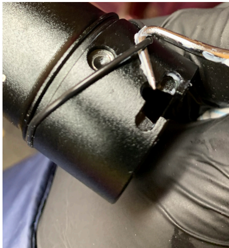
23. Remove the o-ring from the lower part of the post.
