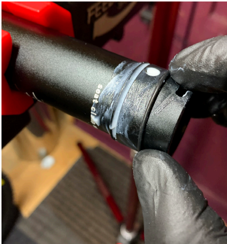
24. Grease o-ring seat and replace o-ring on lower part of post.
