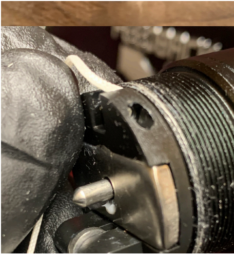
50. Refit the cartridge pin – Note: the rounded end faces outwards.
