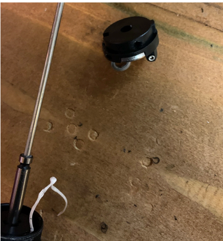
7. Pull pin out from the cartridge – use long nose pliers if you can't grip it with your finger.
