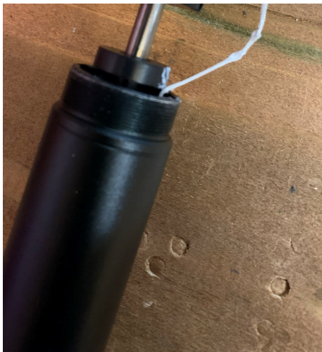
5. Push down on the stanchion to compress the post and reveal the full actuator.
