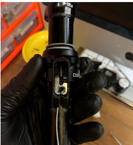
36. Refit string through the collar. Ensure the silver actuator is correctly orientated.
