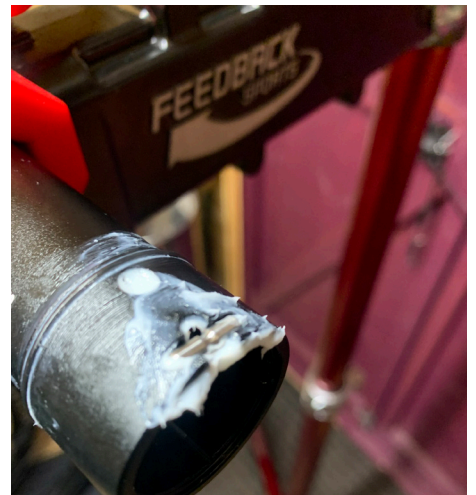
35. Grease and refit silver cable guide.
