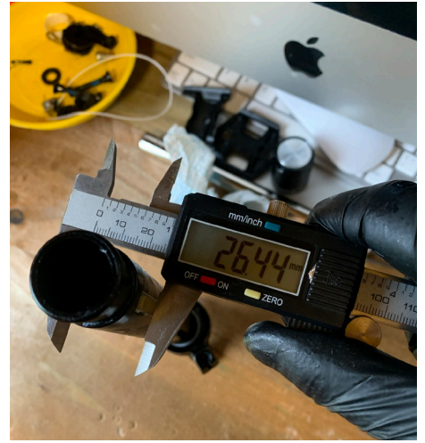
32. Using Vernier calipers measure the diameter of the post around the brass keys to ensure they are fitted correctly.
