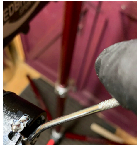
15. Remove the silver cable guide from the lower part of the post.
