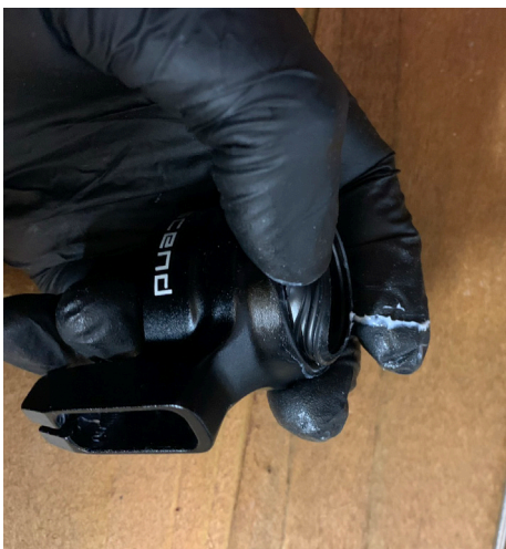
27. Refit seal into collar.
