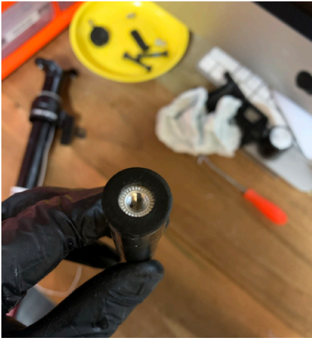
39. Set rubber washer on top of cartridge then side both parts inside stanchion.
