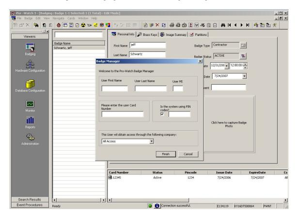
3. From here, the process to add a badgeholder is simple. Enter first name, last name, middle initial if needed, the access cards number, a pin number if you are using one, and finally select the company that will be used to control access of this card.
