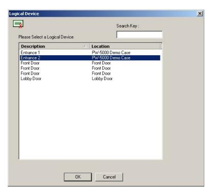
6. Clicking OK will select the reader and close the window. When the window closes another window will open with a list of the available time zones. Select the **time frame** that you want this clearance code to unlock/open the door. Double-click or highlight and click **OK**.
