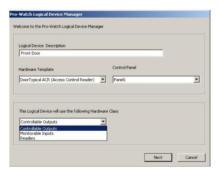
5. This feature is new to Pro-Watch 3.7. When you select the reader address the software will automatically assign the input and output point addresses. These addresses are taken from the hardware point adjacent to the reader port you select.
