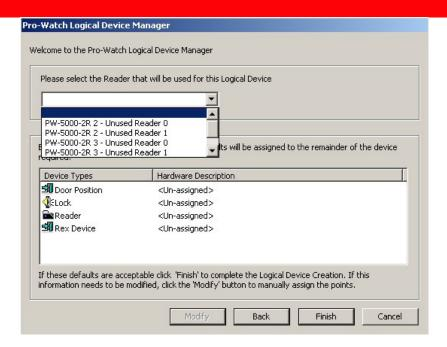
6. In the above example we have selected reader address 0 so the software selected the adjacent inputs and outputs. These can be edited to match your requirements but foreknowledge of this feature will save you time. You can have your hardware installation match the default software assignments.
