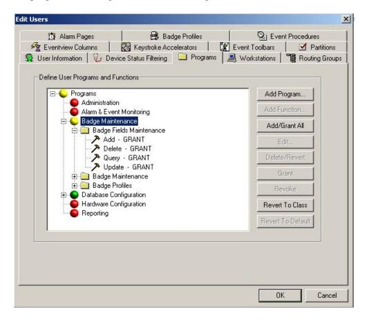
7. Check the rest of the tabs to be sure that this user is configured correctly. Click **OK** to close and save this record.
