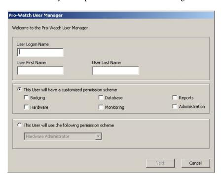
3. The User Logon Name is the name with which the user logs into windows. Make sure your entry is identical to the Windows name. The next two boxes are simply first and last name so you can
