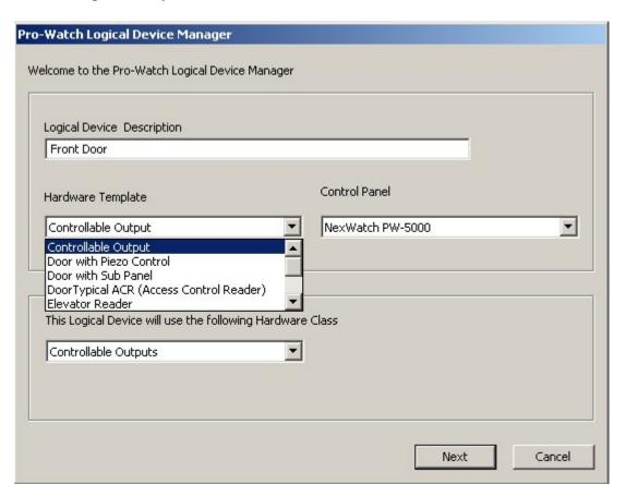
3. Next, select the Control panel to which the device will be connected. If a mistake is made with this selection and the device is created, the only way to correct the mistake is to delete the device and create it again with the proper selections.
