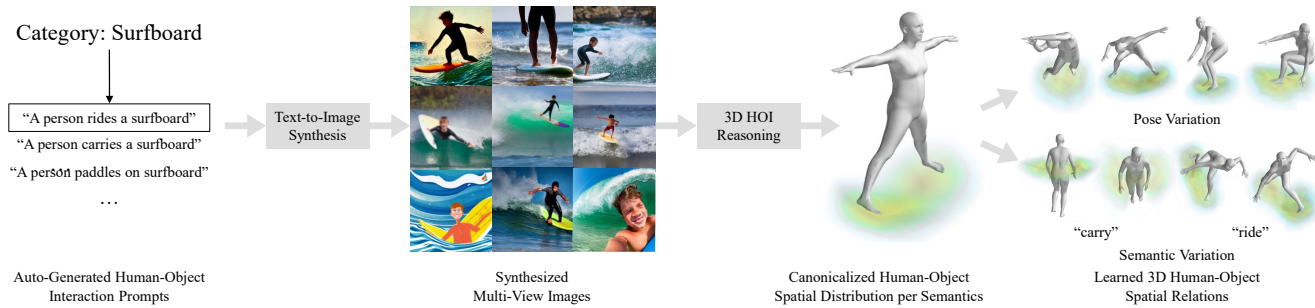
Figure 1. Given an object category, our method, CHORUS , automatically learns human-object 3D spatial arrangements in a self-supervised way. Our method leverages a generative model to synthesize an unbounded number of images to reason about the 3D spatial relationship. As output, CHORUS produces the 3D spatial distribution in the canonical space, which can be deformed for any posed space.
