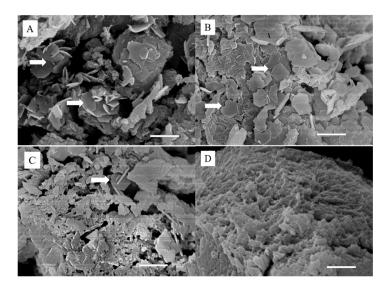
**Figure 2.** The SEM analysis of the surface morphology of (**A**) PAA–0.1M, (**B**) PAA–0.05M, (**C**) PAA–0.025M and (**D**) PAA (white arrows represent simonkolleite crystals, the scale bar: 2 μm).
