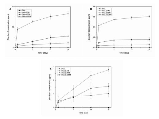
**Figure 3.** The zinc ion release of PAA, PAA–0.1M, PAA–0.05M and PAA–0.025M in (**A**) DMEM, (**B**) PBS and (**C**) SBF after 1, 7, 14 and 21 days, as detected by AAS.
