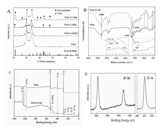
**Figure 1.** (**A**) The XRD patterns of PAA–0.1*M*, PAA–0.05*M*, PAA–0.025*M* and PAA (the simonkolleite spectrum was derived from the standard PDF card No. 00-07-0155); (**B**) The FT-IR patterns of PAA–0.1*M* and PAA: (a) the enlarged view from wavenumbers 1050 to 700 cm<sup>-1</sup>, (b) the enlarged view from wavenumbers 550 to 440 cm<sup>-1</sup>; (**C**) The XPS spectrum of PAA–0.1*M* and PAA; and (**D**) the enlarged Zn 2p and Cl 1s regions of PAA–0.1*M*.
