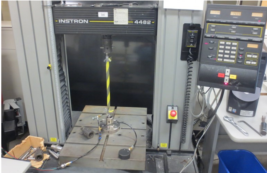
Figure 3-5: PAM cyclic loading set-up
