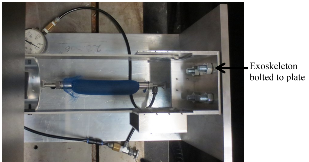
Figure 5-6: Exoskeleton feasibility experimental set-up – top view
