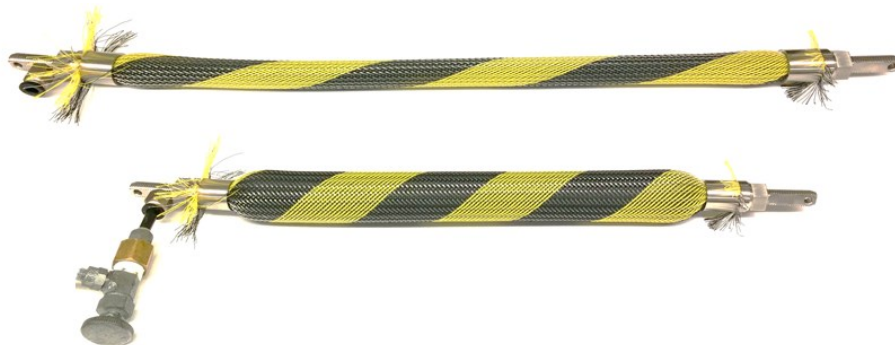
Figure 1-1: Pressurized PAM (top) and deflated PAM (bottom)
