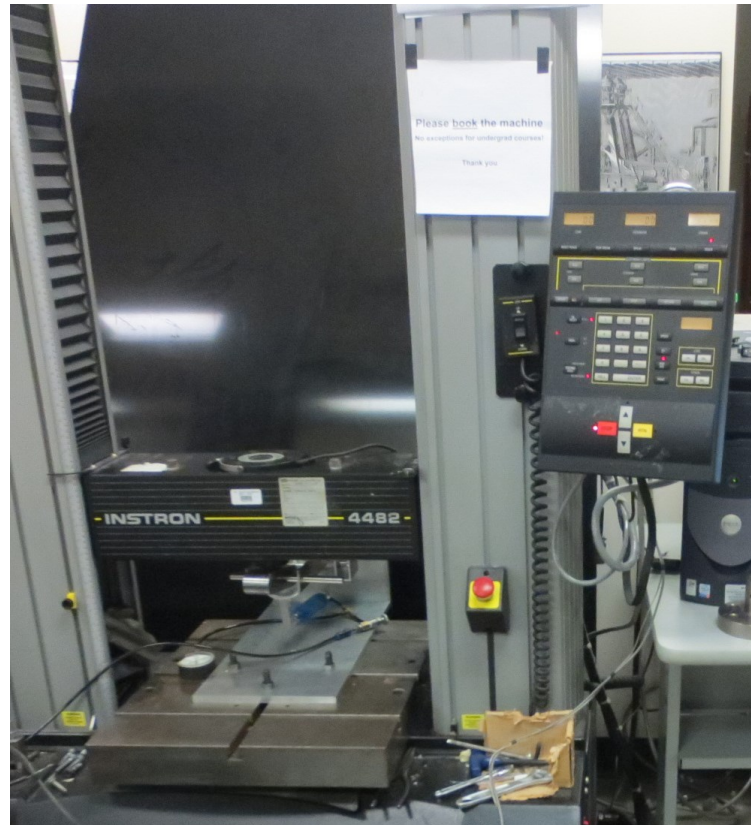
Figure 5-2: Unpowered Ankle exoskeleton prototype feasibility experimental set-up. Jig is attached to the Instron machine with 3 large bolts and the prototype is attached to the jig via large bolts
