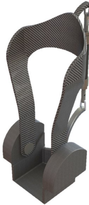
Figure 1-2: Proposed passive ankle exoskeleton
