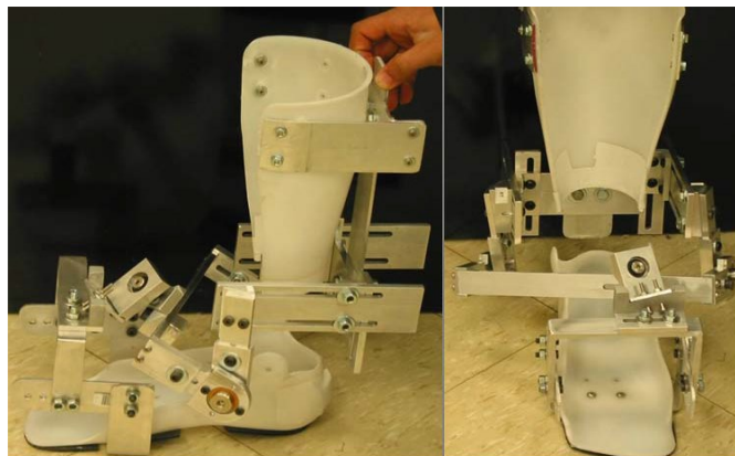
Figure 2-19: Two degree of freedom actuated AFO [59]
