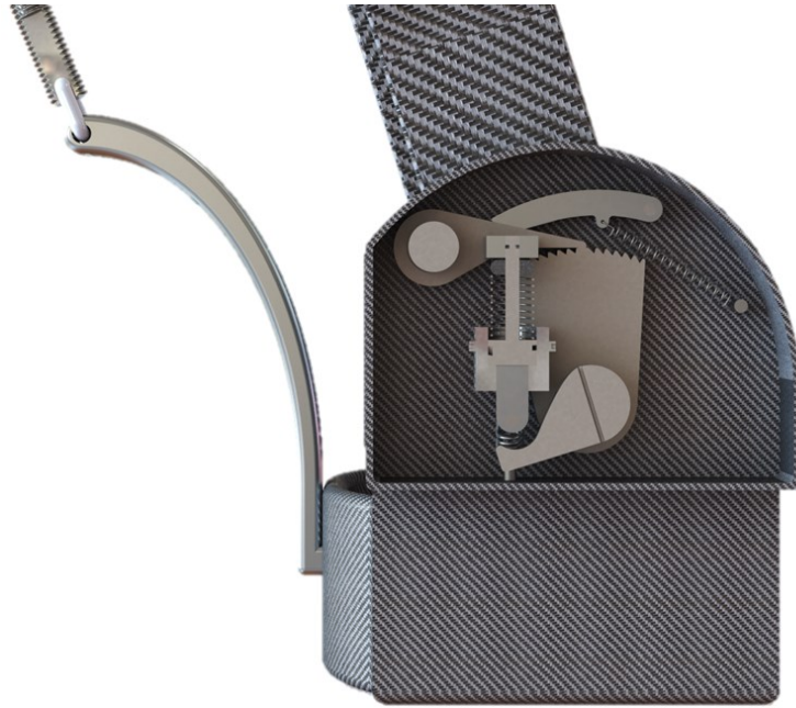
Figure 4-7: Cut-view of timing mechanism
