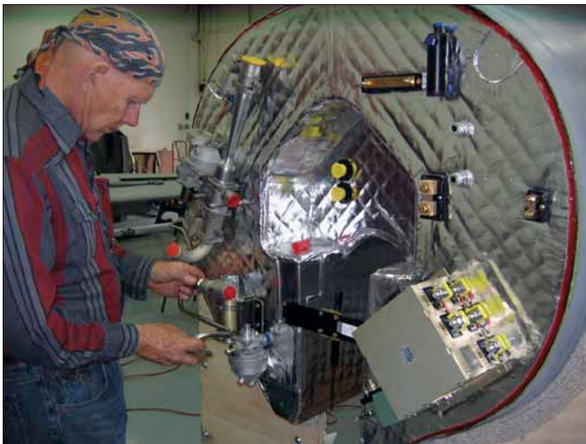
Builder Wendell Solesbee connects a fuel line to the gascolator on the firewall. The firewall blanket protects the composite structure from the heat of a potential engine fire. On Wendell's right is the electrical control unit. In front of him and slightly to his left is the flow pack, which controls turbine bleed air used for cabin pressurization. Other items seen include the brake fluid reservoir, a ground bus bar, and two ammeter shunts.
