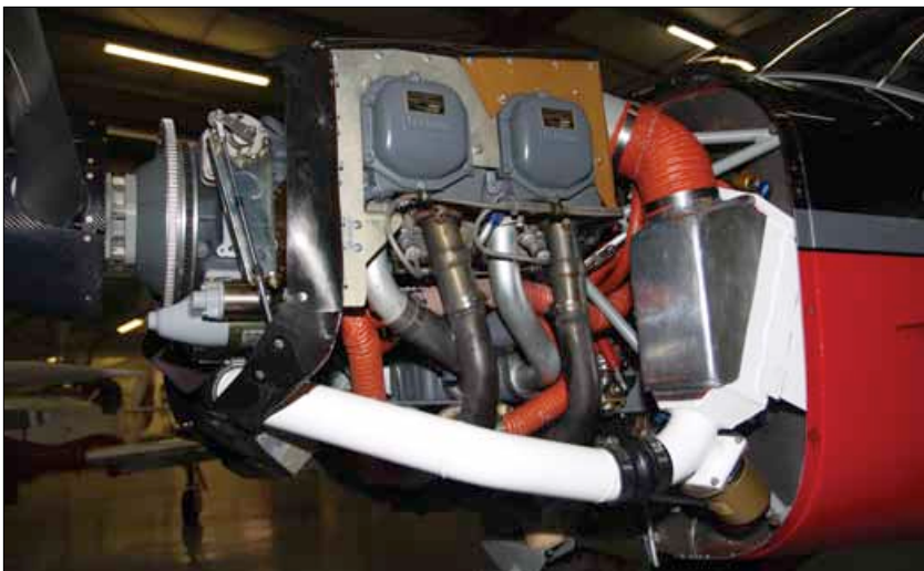
A standard Lycoming IO-360 underpins the turbocharged option. The only internal change was to add nozzles that squirt oil at the bottoms of the pistons.
