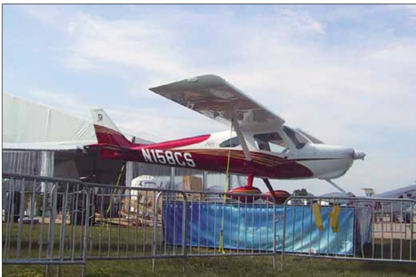
Figure 2. The original tail configuration of the Skycatcher had no fin area below the horizontal tail, and the highly swept-back fin was almost entirely in the "dead zone" above the horizontal tail in a spin.
