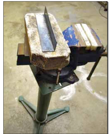
It doesn't take much to practice gas welding: a vise, a firebrick and a couple of scraps of steel.
