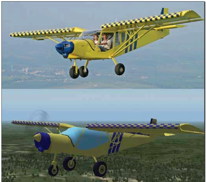
The slat on the leading edge of the wing is an X-Plane "misc body." It is specified to have zero drag and does not participate in the aerodynamics of the wing itself.
