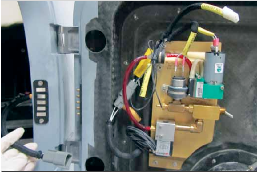
To properly seal each door to an airtight condition, a small pump provides pressurized air to inflate the seal around the door. Electrical contacts in the door jamb allow power to be connected to the pump and controlled from the instrument panel.
