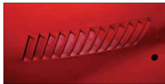
Twin louver sets increase the flow of cooling air for the turbo installation.
