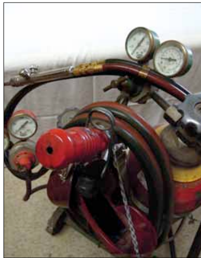
A pair of regulators with gauges controls the flow of gasses to the torch. Red is acetylene, green is oxygen.
