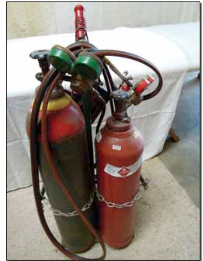
One of the beauties of gas welding is that it's self-contained. Everything you need—gas, goggles, igniter, torch—is on one wheeled caddy.
