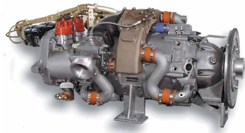
The aircraft version circa 2001, showing most of the major accessories installed except for the exhaust system, spark plugs and fuel-injector lines. It was FAA certified in 1957 with only one spark plug per cylinder.
