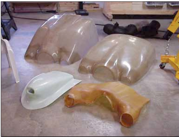
The raw materials: a top and bottom cowling, air scoop (white) and a plenum (orange), ready for the builder to trim and fit, and then trim and fit again. Eventually all will fit this custom installation. Then let the riveting, bonding and bolting begin!
