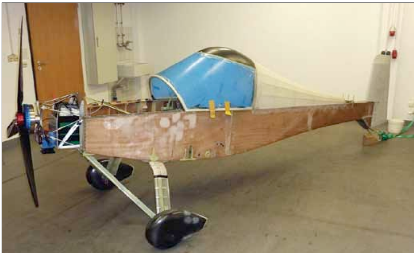
MC-30 in LSA's workshop, showing simple construction, motor and battery installation. This was designed by a Concorde designer.
