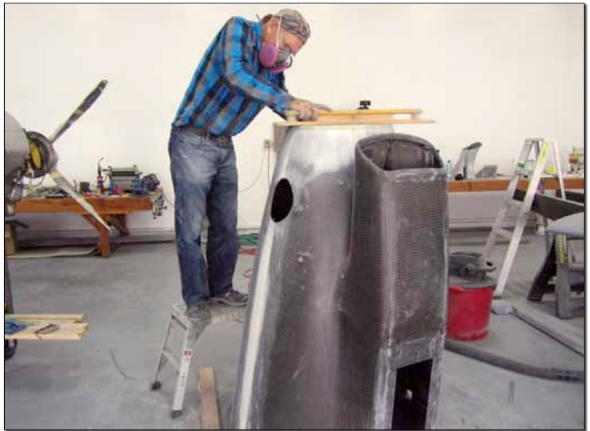
With the engine and propeller now in place, Wendell can bring his considerable expertise with composites to bear on fitting the cowl. This was the most difficult composite work to be performed on the Evolution. It is also one area where an inexperienced builder would need some serious help.
