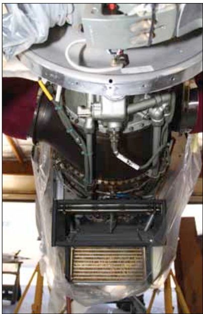
The engine air intake mates to the scoop on the cowl. Inside the cowl the air is split so that some of it goes to the oil cooler, seen below the engine air intake, with the rest going into the engine. The plastic is there to keep dust out of the engine while the Solesbees sand the fuselage.
