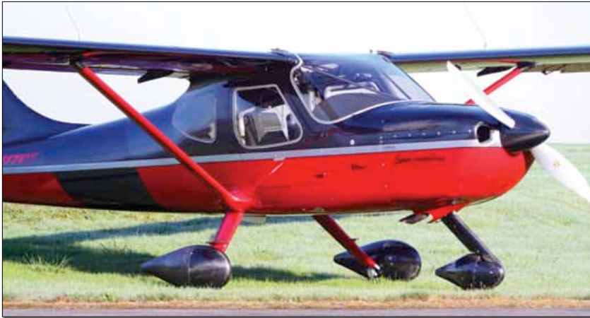
From across the ramp, the Sportsman TC belies its new skin through a cosmetic treatment. Although it's lighter, the carbon-fiber skin appears the same as the regular fiber-glass it replaces.
