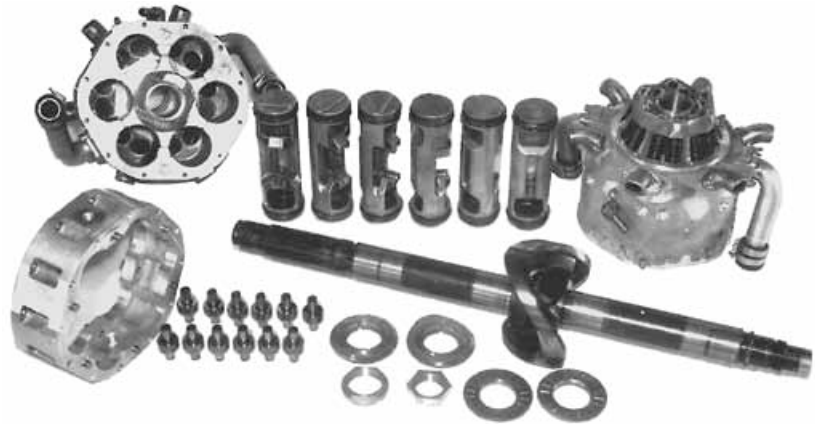
A closer look at the main engine components. Twelve cylinders and six double-ended pistons turn the center shaft via roller bearings, with substantial thrust bearings on both sides of the center cam.
