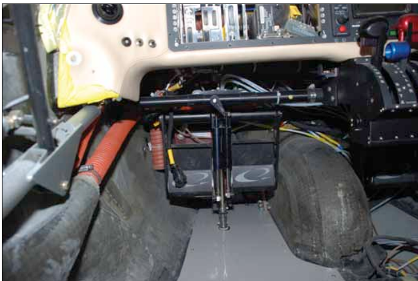
A small hand crank makes adjusting the position of the rudder pedals easy. In a matter of seconds, a taller or shorter pilot can be made comfortable with a few simple adjustments.
