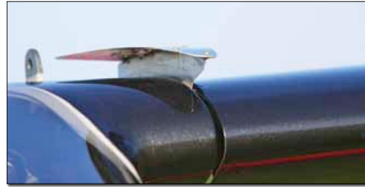
Vortex generators inboard and ahead of the ailerons help condition local flow to improve low-speed handling. The Sportsman, given its size and wing area, has exemplary low-speed manners.
