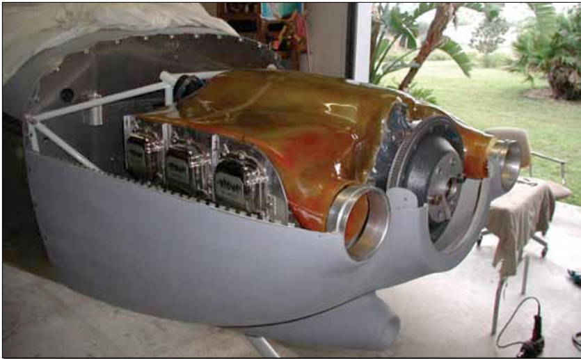
Here is the original configuration with 4-inch intakes.
