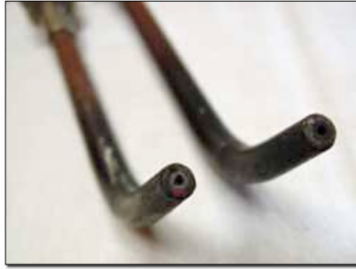
Torches come with different orifice sizes. Thicker metal requires more heat and more fuel to create the weld.
