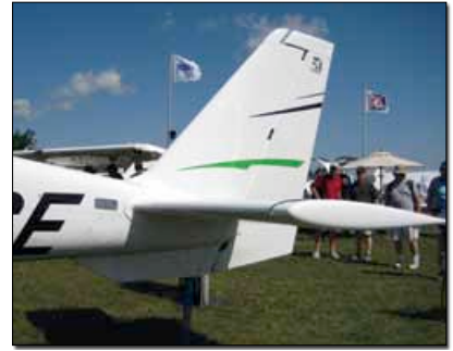
Figure 3. The tail configuration of the definitive production Skycatcher. The rudder now extends below the horizontal tail, and some ventral fin area has been added.
