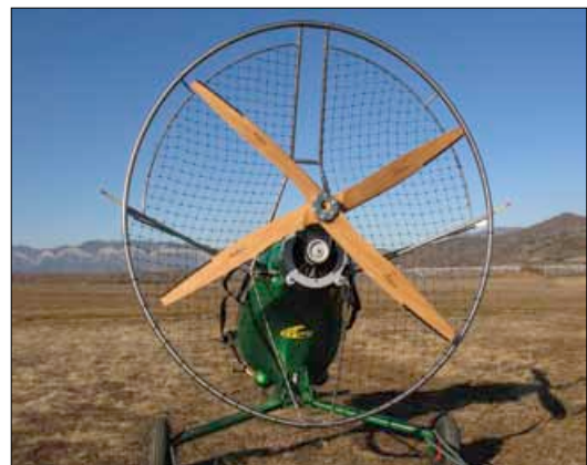
E-Fenix shows a four-blade E-Prop with offset blades. These cause "dephasing of sound waves and lower noise."
