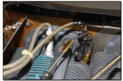
New fuel injectors include pressurized shrouds to ensure that the injector body is always at a higher pressure than the intake manifold.
