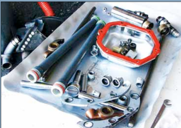
Trays are good for keeping all of the parts together during disassembly and reassembly. They can be marked to indicate the proper orientation of parts.
