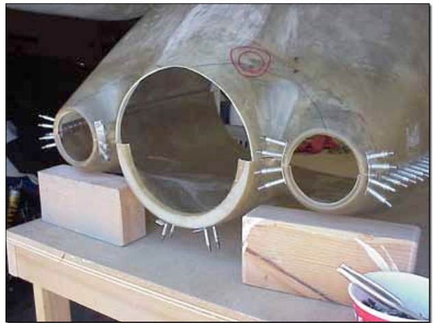
This is the best time to decide how large you want your air intake openings. It's easy to trim the openings to an exact size and fit the rings before the final sanding and filling.
