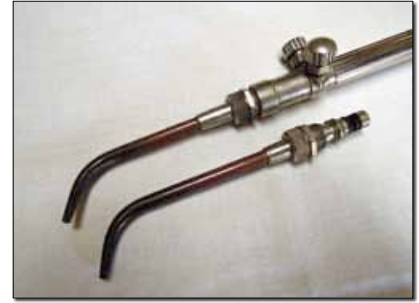
Interchangeable torches mix the oxygen and acetylene and fit comfortably in hand.
