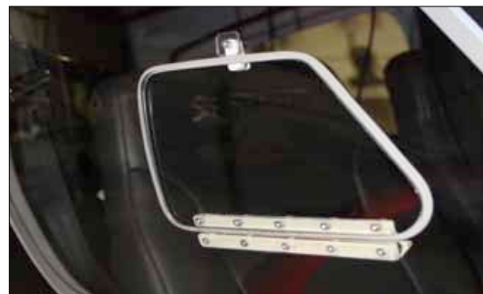
A new optional opening window can be used as a camera port.
