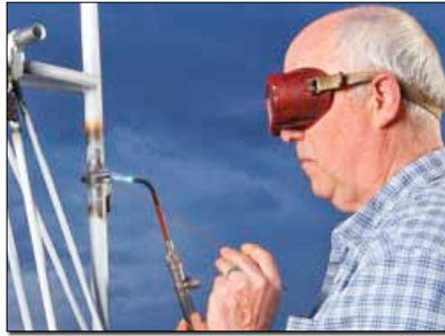
Groelz adds a tab to the tailpost of his Christavia fuselage.
