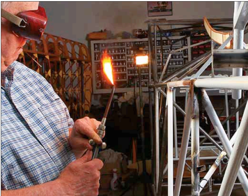
When the torch is first lit on acetylene alone, it generates a soft yellow flame.
