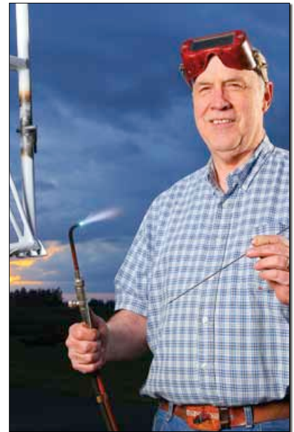
When the oxygen valve on the torch is opened (slowly) the flame turns into a lovely blue cone.
