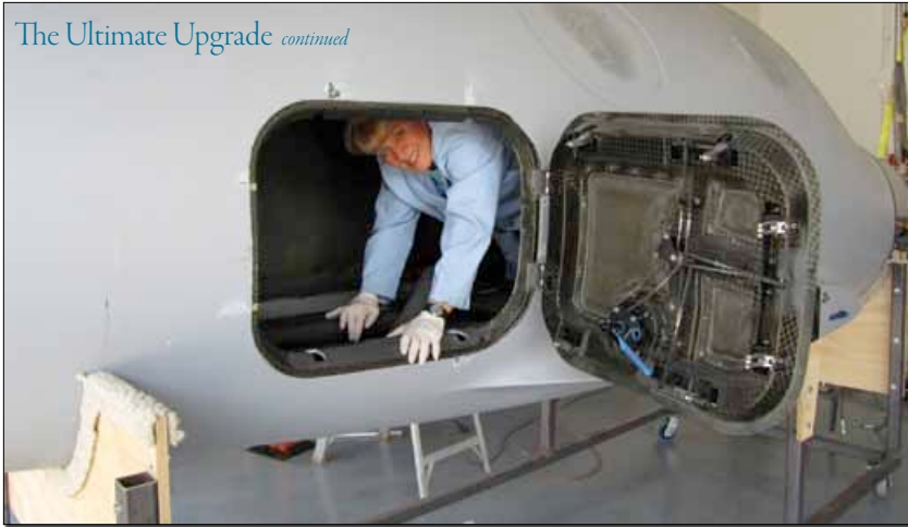
Martha Solesbee glasses in partitions in the cabin floor. These compartments will house various items such as the landing gear hydraulic system, the emergency oxygen system, and a number of electrical components. The complex latch hardware can be seen on the baggage door.
