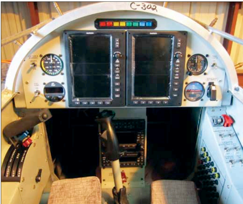
Good judgment in design can be shown when planning backup instruments to cover potential failures.
