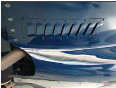
An example of louvers appended to the bottom of an RV-10 cowling to help draw out the hot air from the lower cowl.
