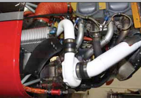
The Garrett turbocharger resides below and behind the engine on the copilot's side. A heat shield keeps the oil cooler (on the firewall) from picking up infrared heat.
