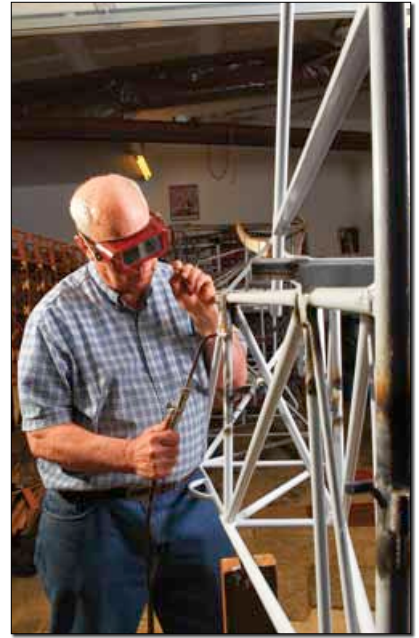
The fuselage was gas-welded from plans.
