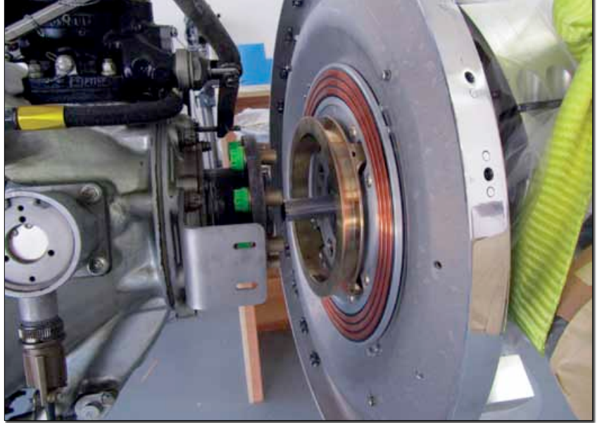
The contactor ring on the back of the prop allows for electrical power to be transferred to the propeller heating (deicing) elements. Access to the prop bolts becomes limited where the prop and engine come together. Wendell had to fabricate a special tool to tighten these bolts.
