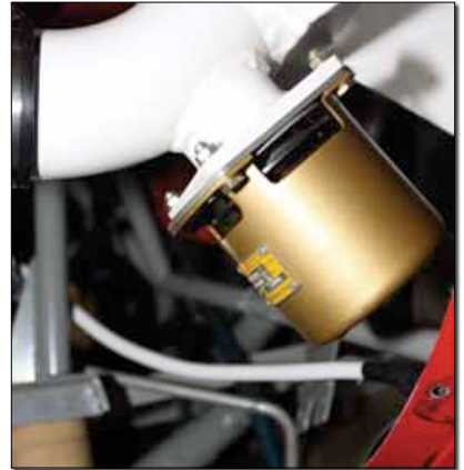
Although the better turbo systems use automatic wastegates, they all need a so-called popoff valve to prevent overboosting of the engine in the event of a controller or wastegate failure.
