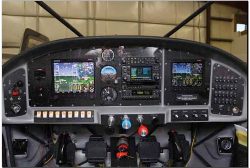
This high-end IFR panel includes dual Advanced Flight Systems EFISes along with analog backup gauges and an AFS-branded, TruTrak-built autopilot.
