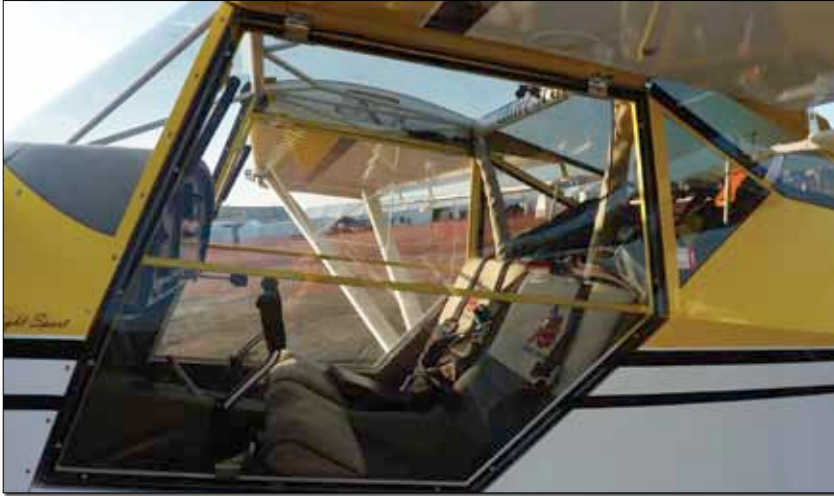
A full-Lexan door means that this Kitfox 7 is an excellent observation aircraft. The fact that it can safely fly at speeds as slow as 30 knots helps qualify it, too .
