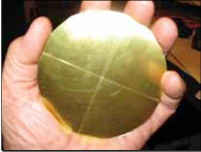
A perfectly circular ground plane.
