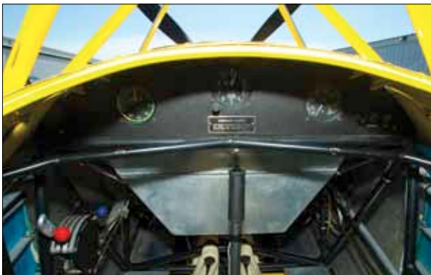
The front instrument panel is typically sparse, which may necessitate cooperative communication with the back-seater.
