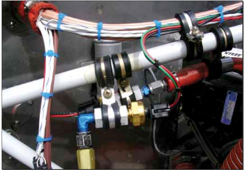
Note the usage of cushion clamps and high-temperature Tefzel ties in this installation.
