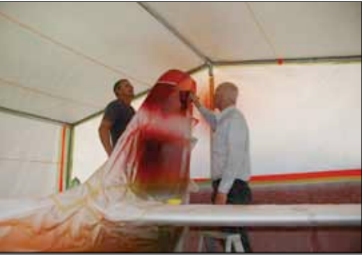
With the masking removed, Wendell and Terry inspect their handiwork on the tail of the Evolution. Terry will follow up with striping and shadow details later.
