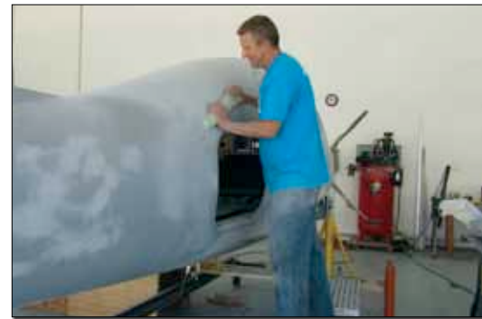
Terry Solesbee block-sands and fills the fuselage after the first coat of primer to smooth the high spots left from the manufacturing and assembly processes. He is using a flexible long board to better conform to the continuous curves of the Evolution.
