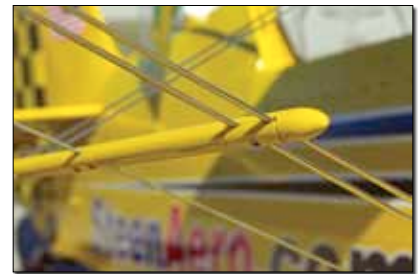
Note the redundant flying wires, standard on aerobatic biplanes.
