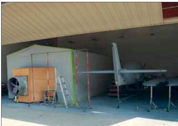
The Solesbees rented a portable booth to paint the Evolution. It fit well in their hangar at the Chino airport. The booth itself is made of plastic sheeting over a pipe framework. Note the large fan box on the end near the outside.
