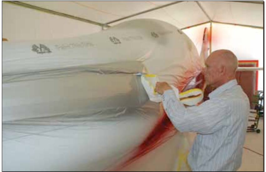
Wendell removes the masking from a section of the fuselage. With the slow-drying water-based paints used for the colors, it is important to be patient while unmasking. It would be a shame to rush at this point and have to redo so much hard work.
