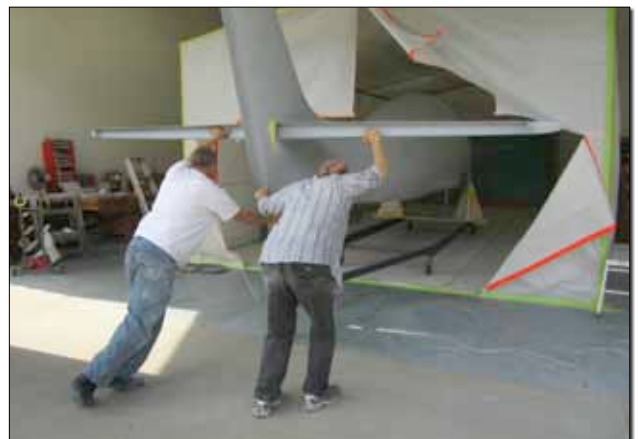
Wendell and Terry load the Evolution fuselage into the paint booth. Once the plane is inside, the fan box simply wheels back into place. The dolly that Wendell welded together makes moving the big Evo fuselage easy for two people.
