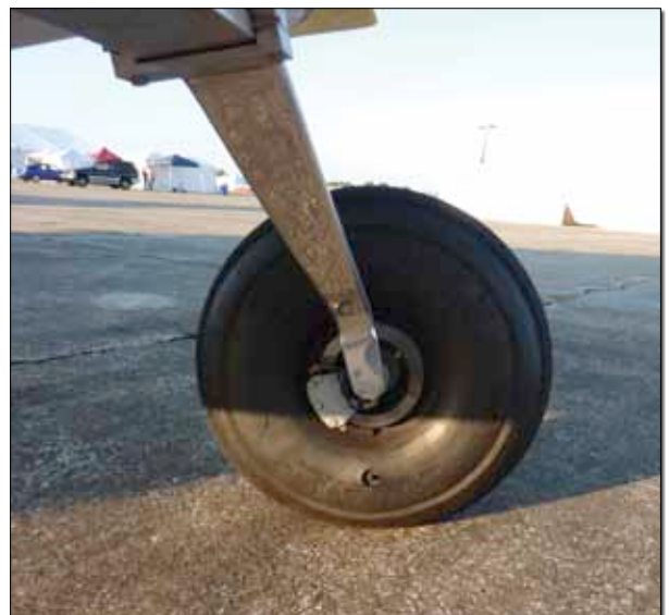
The Grove landing gear on the Kitfox line of aircraft is made from sprung aluminum. It's light, but it can take the beating of off-field landings.
