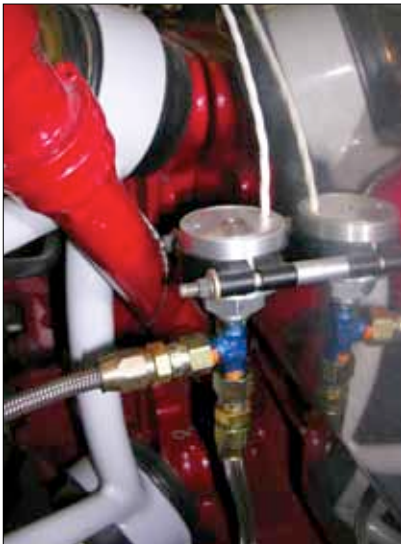
Standoffs may be used to better position some sensors and probes.
