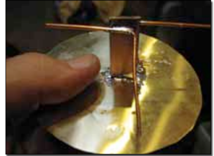
The antenna on the ground side of the microstrip.
