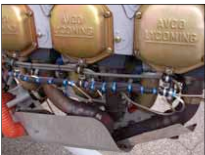
More high-temp Tefzel ties and protective coverings used for wires near the exhaust.
