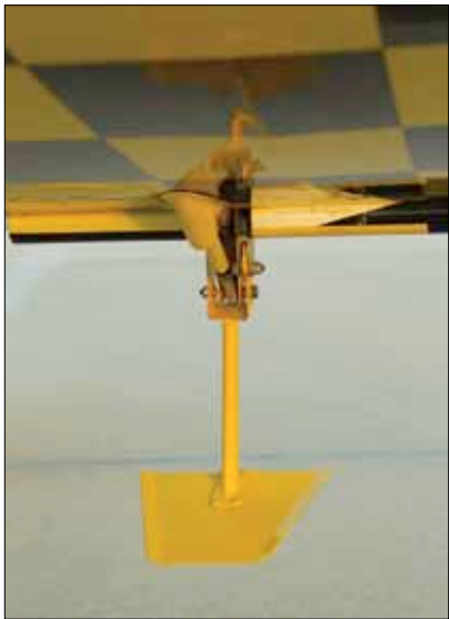
Aileron spades. They may not be necessary, but the ailerons had a great feel with them.
