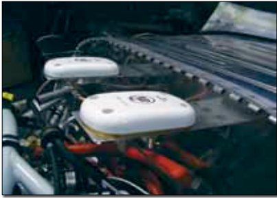
Antennas mounted forward of the firewall need to be adequately secured and grounded.
