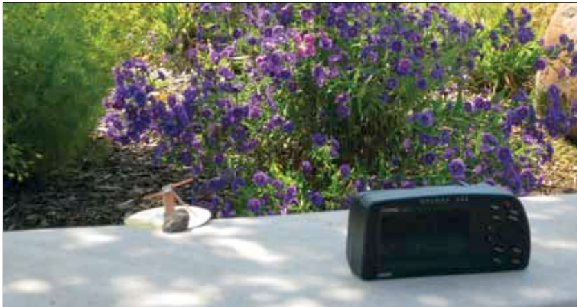
The antenna pattern range at Sierra College. The rock on the ground plane provides extra stability.
