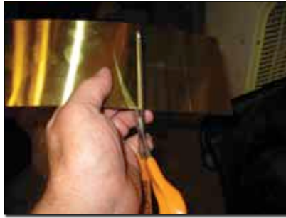
Carefully cutting the ground plane with kitchen shears.
