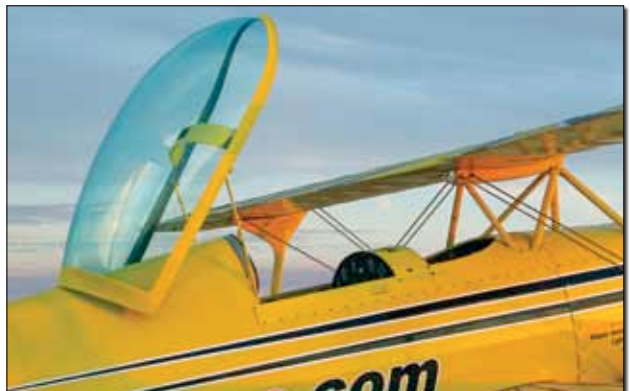
The canopy arrangement is unique, and the canopy can only be released from the back seat.
