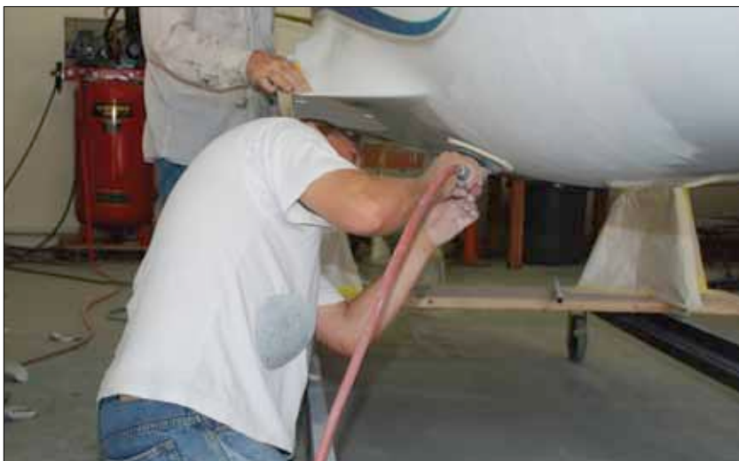
Sanding, sanding and more sanding. That is what painting is all about. Before the clear coats go on, the entire fuselage is lightly sanded to remove any small imperfections and ensure a good grip for the next layer of paint.
