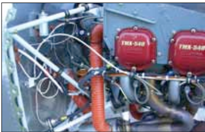
You can see some of the many wires that will be on the firewall as well as running throughout the engine compartment.
