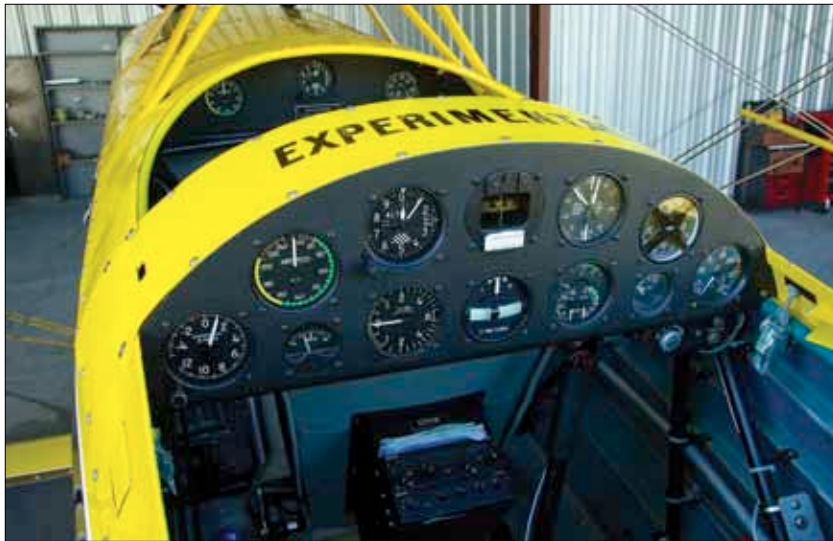
Yellow Bird's rear instrument panel. The airplane is normally piloted from the back seat.
