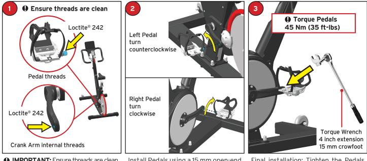
IMPORTANT: Ensure threads are clean using 50/50 isopropyl and water mix. Allow the area to dry completely before application.
