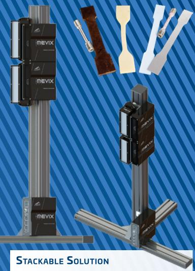
The MEVIX camera modules can be stacked up to **extend the Field of View** without losing the **desired resolution**. This option brings ability to measure long or high elastic samples with high accuracy.
