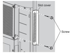
2 Insert the terminal board to the main unit slot, and tighten the 2 screws.
