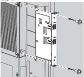
• Tightening torque guideline: 0.5 N·m or less
