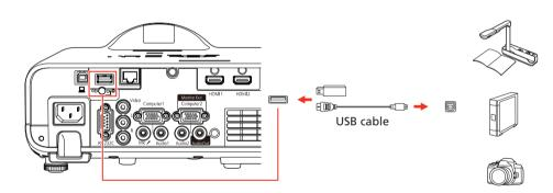
If you connect a digital camera, USB flash drive, or USB storage device, you can use the projector's PC Free feature. See the online *User's Guide* for details.
