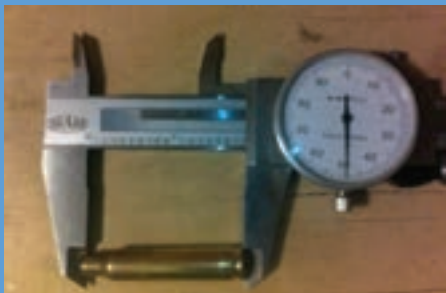
Note that the ADI cases have been trimmed to the same length. Trimmed length = 1.749" or 44.425mm
