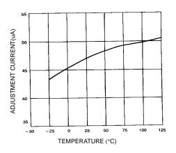
Figure 2. Adjustment Current
