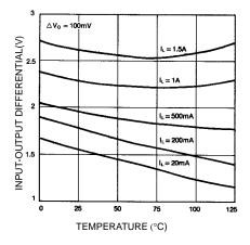
Figure 3. Dropout Voltage
