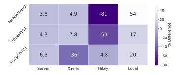
Fig. 9. Inference time differences (%) between Basic and Extended optimizations across devices, with native models from PyTorch.
