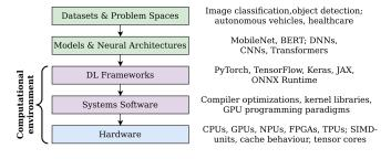
Fig. 4. Relevant layers in the deep learning systems stack [11].
