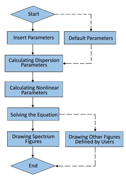
Fig.2-3 Structure of Simulation Program
