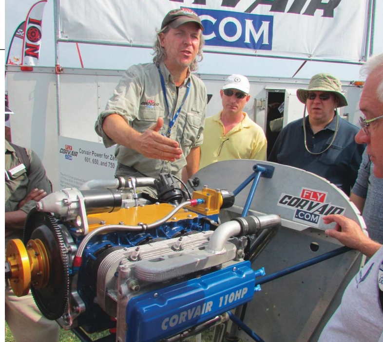
William Wynne has educated people to the fact that they can make an O-200 class engine for a fraction of the cost. William's conversion package is based on the Corvair engine of the 1960s.
