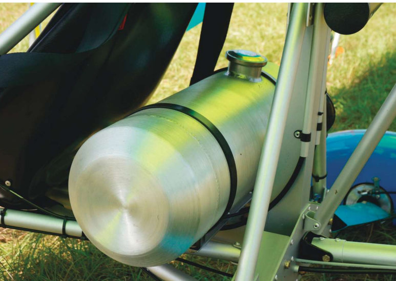
This elegant, 5-gallon, spun-aluminum fuel tank is from a sandrail buggy.
