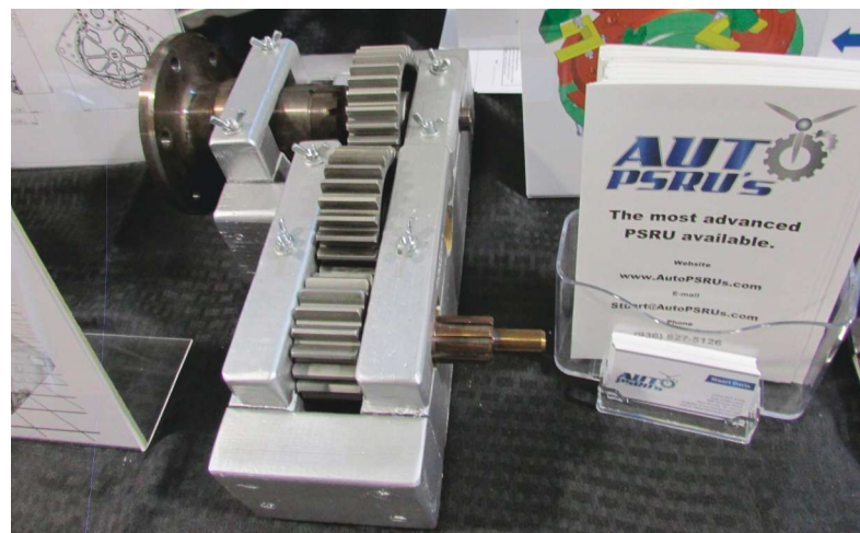
AutoPSRU's offset up gearbox is quite compact and has a complete oil system, including an optional prop governor.
