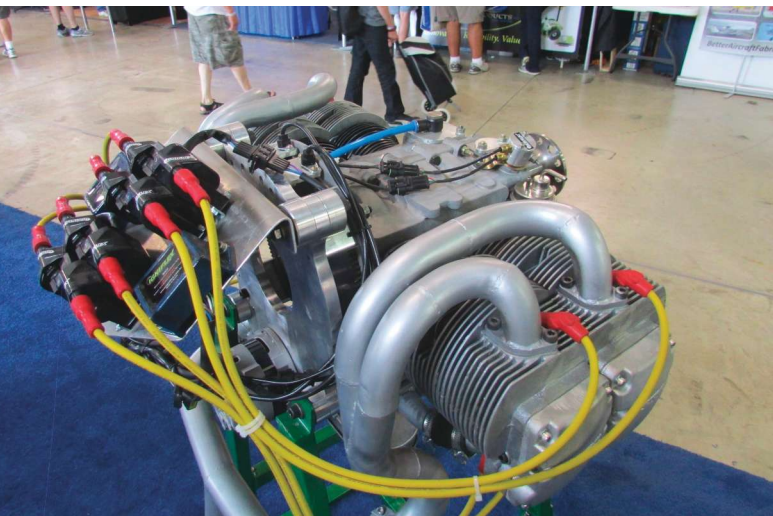
Motorav has beefed up its VW-based engine components. The normal VW heads are considered to be under-finned; Motorav has addressed that as you can see.
