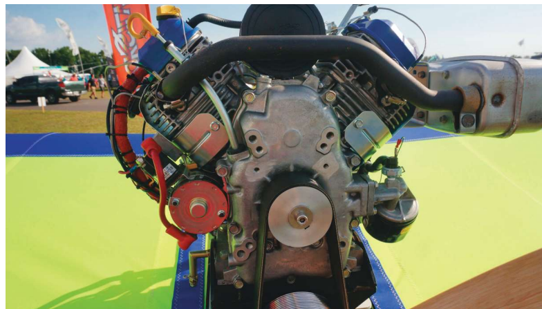
A four-cycle, V-twin Briggs & Stratton engine on the Aerolite 103, shown here at Sun 'n Fun, is now mounted under the wing, according to reports on the Aerolite Facebook page.
