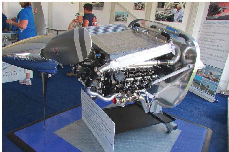
The 350- to 400-hp plus EPS Diesel is the wave of the future for the heavier end of light planes. It is only a bit heavier and more expensive than a gas engine, but it has a much lower fuel burn of a less expensive fuel. Comparable turboprops are lighter, much more expensive, and use twice the fuel.
