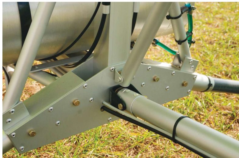
The Aerolite 103 features robust aluminum tube-and-gusset construction in the landing gear area.
