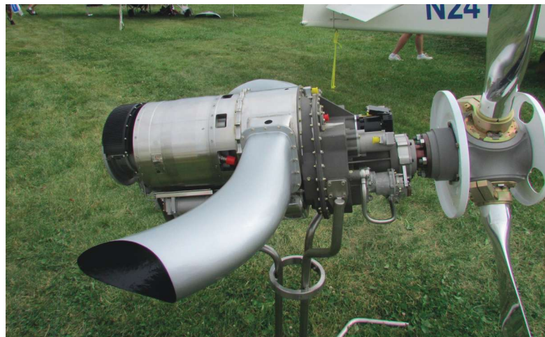
This tiny, 240-hp turboprop from PBS is being tested in the RV-10 shown behind it. If you have the money for the engine and fuel, go for it.
