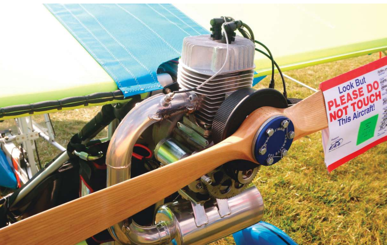
The underwing mount for the Hirth F-33 with a cog belt updrive and electric starter.
