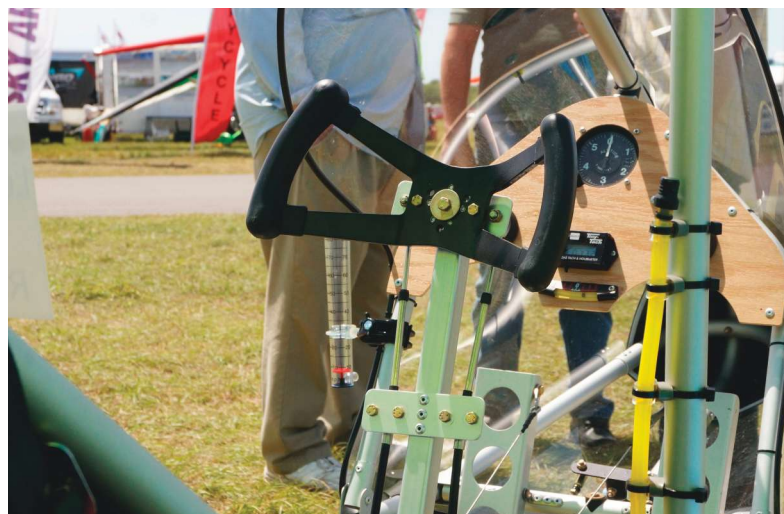
A view of the cockpit, control yoke, and the push-pull control cables.
