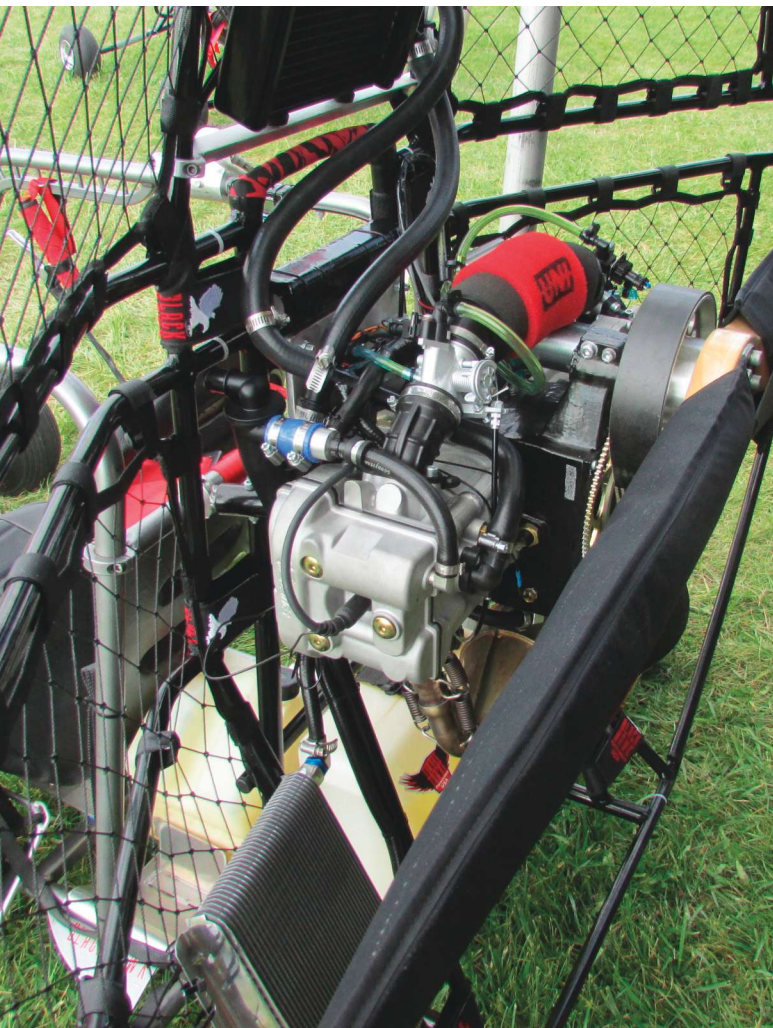
The Verner JCV 360 is a compact, liquid-cooled flat twin four-stroke engine of 35 hp and 60 pounds. It is successfully flying some single-place light aircraft such as powered parachutes.
