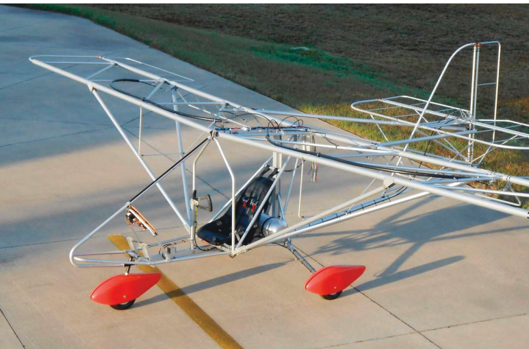
A bare Aerolite 103 fuselage with the control system installed.
