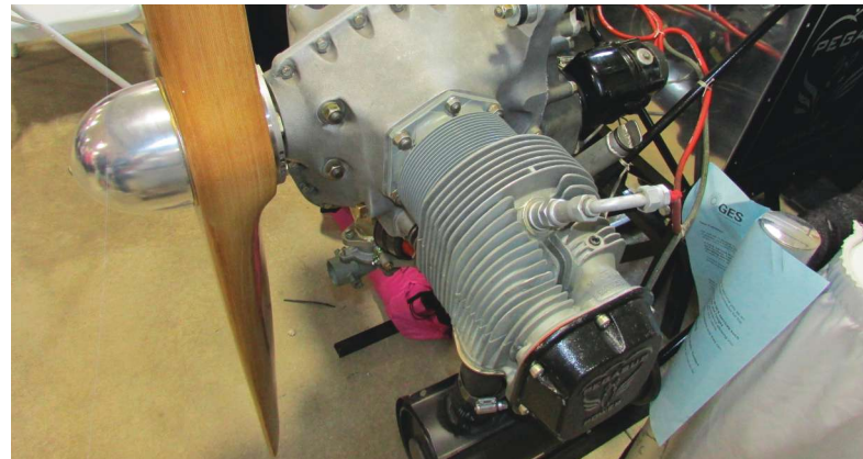
Pegasus Power has a kit of special parts to make a 60-hp, O-100 flat twin engine using O-200 cylinders and components. The custom crankshaft and lightweight rods and pistons make for a smooth-running engine as demonstrated at EAA AirVenture Oshkosh 2014 in the Ultralight/Lightplane area.
