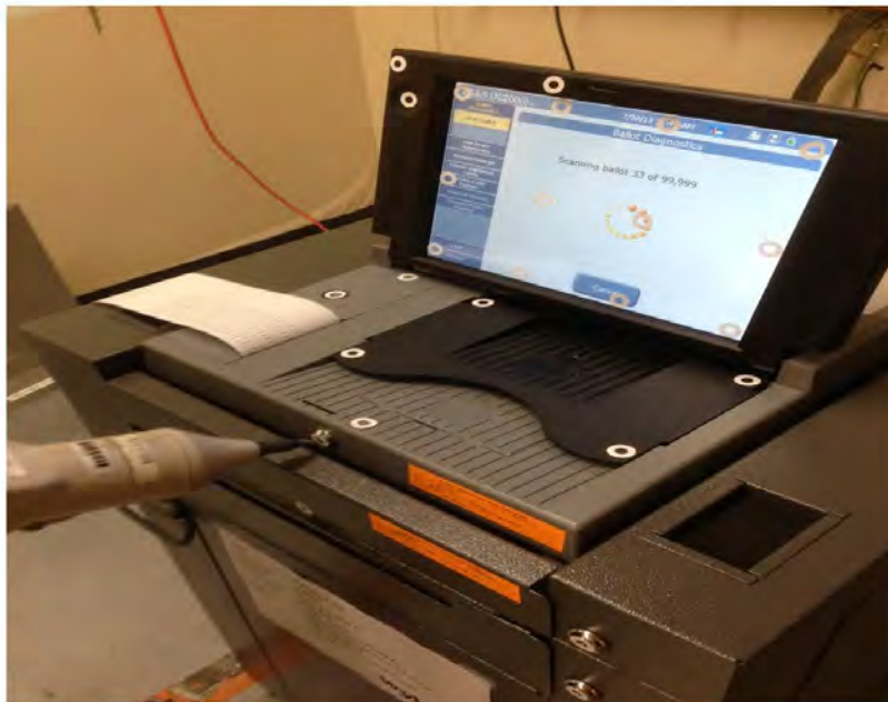
Photograph 18: ES&S FL EVS 4.5.0.0 Electrostatic Disruption
