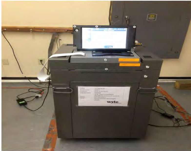
Photograph 17: ES&S FL EVS 4.5.0.0 Electrostatic Disruption
