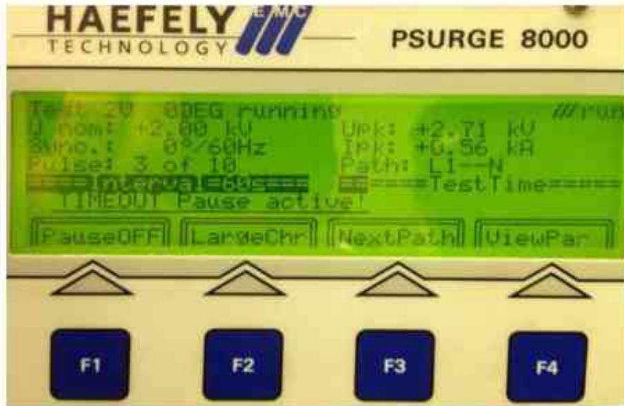
Photograph No. 11: ES&S FL EVS 4.5.0.0 Lightning Surge
