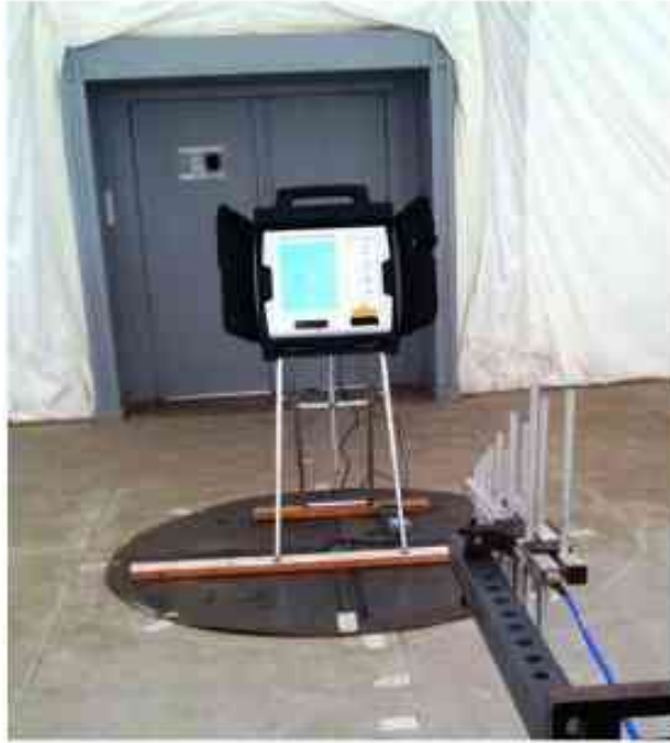
Photograph No. 15: ES&S FL EVS 4.5.0.0 Electromagnetic Emissions
