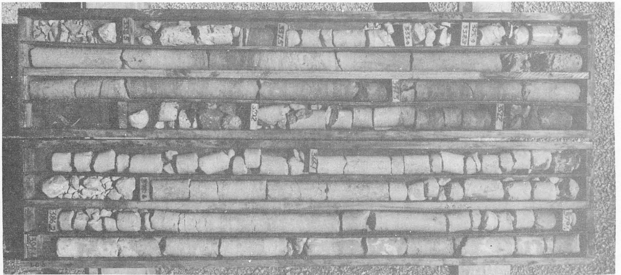
Box 14 and 15; 321.5 to 394.6. Core reduced from 6" to 2". Depth increases from upper right to lower left. Used rock bit from 317.9 to 321.5 and from 325.9 to 332.3. Generally very poor core recovery. Note scattered chert from 359.2 to 360.3.
