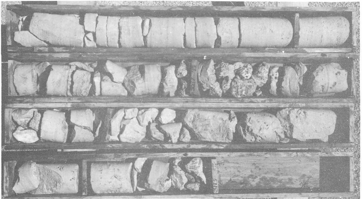
Box 10 through 13 ; 298.9 to 317.9. Rock bit used from about 296.3 to 298.9. Rock is very hard and generally highly fractured and solutioned in last three boxes.
