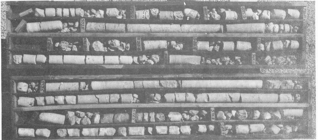
Box 20 and 21; 484.2 to 593.3. Very heavy core loss in this interval. Core in box 20 represents all that was recovered in 66.7 feet of hole. Highly solutioned with cavities up to 2'.
