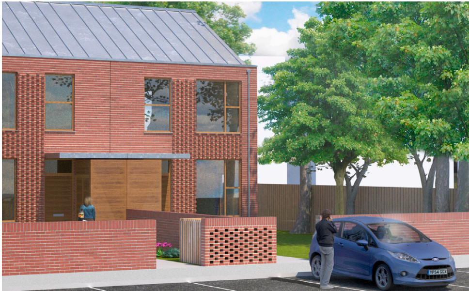
Example where storage is integrated into both the boundary wall and porch using complementary materials
