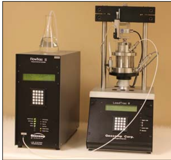
Figure 5. Front view of a fully automated constant rate of consolidation system.
