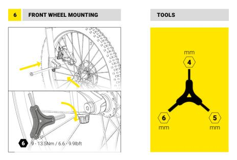
1. Guide your wheel into the fork and guide the rotor between the brake pads.
