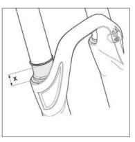
Set the O-ring (sag indicator) at the bottom of the fork stanchions. Dressed in full riding gear assume normal riding position on the bicycle. Step off the bicycle and measure the distance the O-ring (sag indicator) has moved. Sag should be set to approximately 10-15 % of the fork travel.
