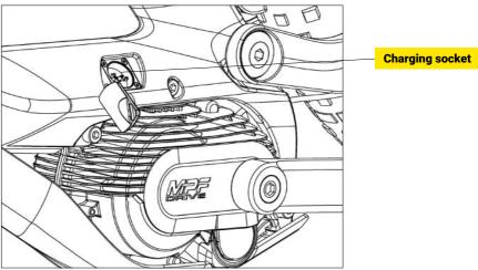
Plug the charger plug into an appropriate AC outlet (depending on the charger) using the appropriate plug/adapter for your country's standard.
