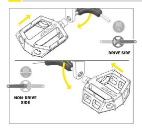
1. Take the pedals out of box, grease the thread and tighten them using the tool (three-arm hex key number 6) (see picture above).
