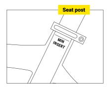
The saddle height is always measured with the crank arm pointed down and in line with the seat tube. The distance from the centre of the pedal axle to the top of your saddle is your saddle height. Before changing the height of your saddle, you should measure your current saddle height.
