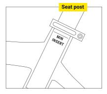
To lower the saddle, weight the saddle firmly with your hand or sit on the bike while pressing and holding the actuation lever or remote. Release the lever when the desired height is reached.
