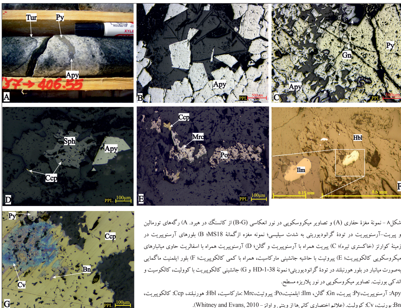
Figure 8. Drill core specimen (A) and reflected-light microphotographs (B-G) from Hired. (A) tourmaline and pyrite-arsenopyrite veins in highly silicified granodiorite; core sample from borehole- MS18; B) arsenopyrite crystals in quartz matrix (dark grey); C) pyrite associated with arsenopyrite and galena; D) arsenopyrite, and sphalerite containing microscopic inclusions of chalcopyrite; E) pyrrhotite replaced at rims by marcasite, associated with minor chalcopyrite; F) ilmenite occurring as inclusion in hornblende in granodiorite body; sample HD-1-38; and G) partial replacement of chalcopyrite by covellite, chalcocite and minor bornite. All microphotographs in plane-polarized light.
