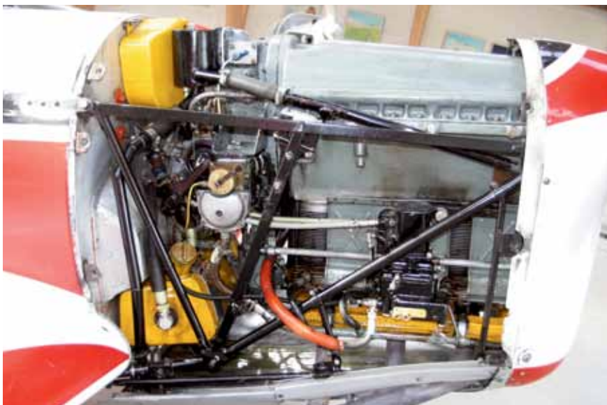
The Gipsy Major engine chosen to power the KZ VIII gives the airplane a decidedly Chipmunk look.
