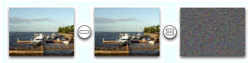
Figure 4.2: The input image I (leftmost) and its perturbed version T(I, 75\%) (middle): differences are not visible by the naked eye. However, they are present in the LSB channel (rightmost).
