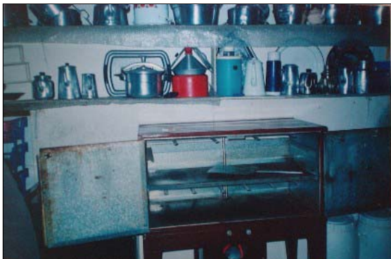
Fig. 23. Gas ovens, provided in Phase II, reduce reliance on fuelwood. Instead of having to gather firewood daily, village women now collect wood only once every two days. Gas, however, is expensive.
