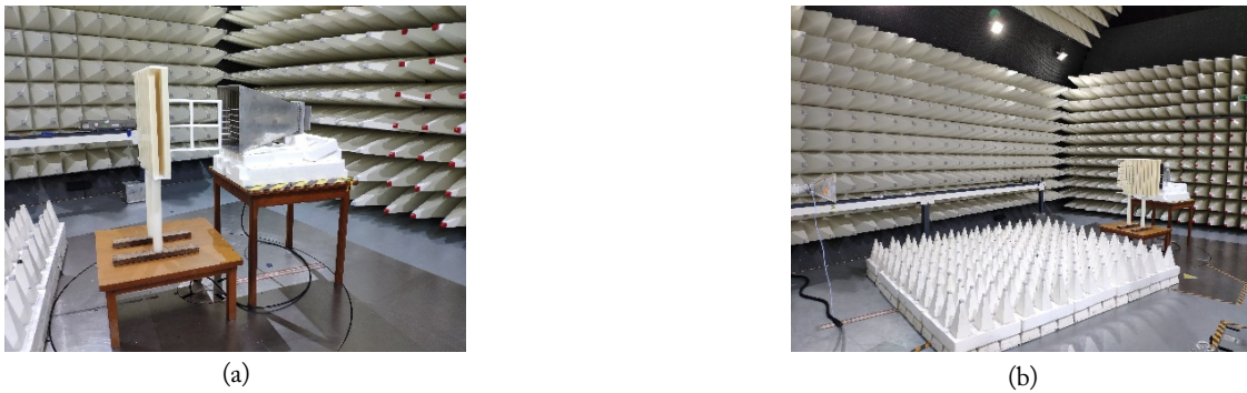
Fig. 16. The measurement setup for fabricated hybrid metamaterial with an asymmetric horn antenna in anechoic chamber: (a) side view and (b) perspective view.
