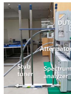
Fig. 2. Measurement setup for the impedance mismatch effect between DUT and the measurement system. The impedance stub tuner is attached to the input port of the spectrum analyzer to produce arbitrary impedance matching status.
