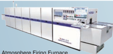
Atmosphere Firing Furnace (HSA 1508-0611NH Belt Furnace)
