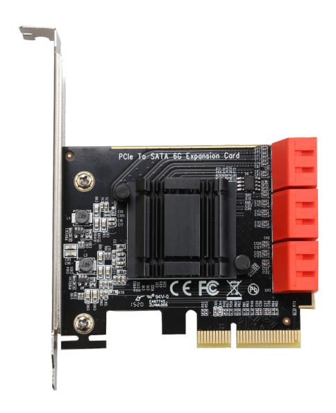
The TXB113 is 6-port SATA III (6 Gbps) to PCI Express x2 Gen 3 Host Card. It adds 6 AHCI SATA III port to computer though a PCIe slot (x4), delivering multiple internal 6Gbps connections for high performance hard drives and Solid State Drives (SSDs).
