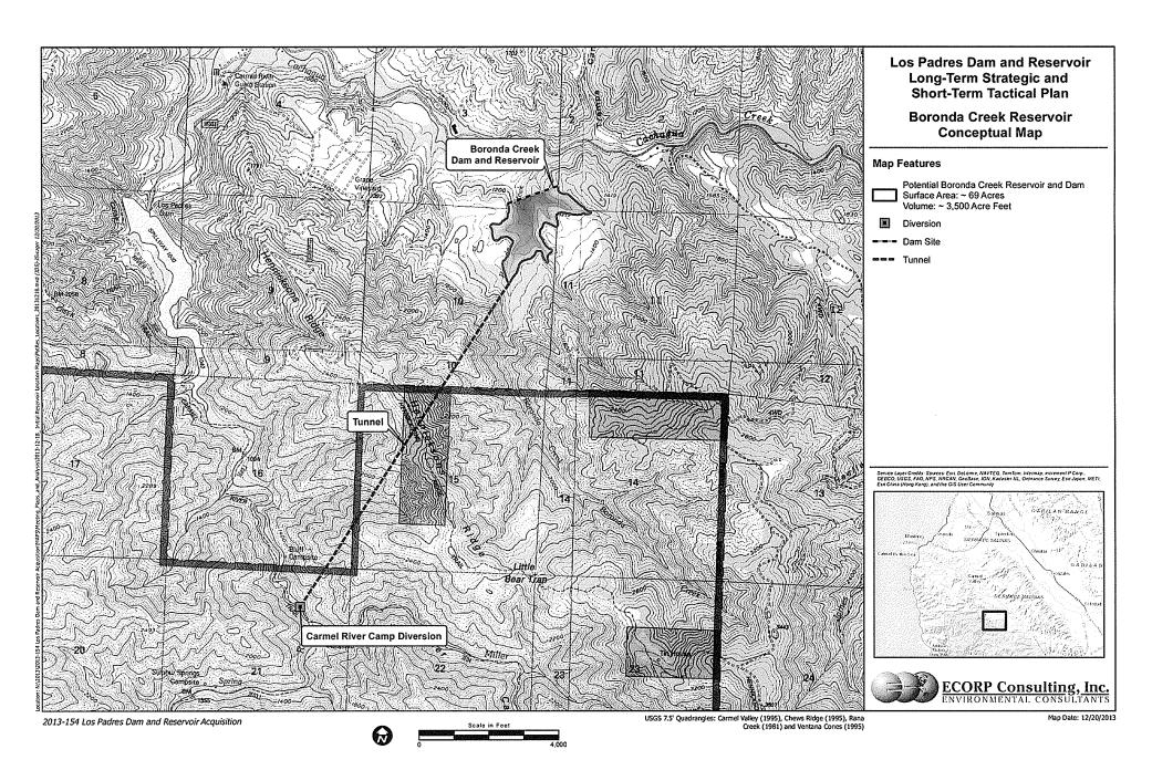
suggest that a concrete lined tunnel of about 4 feet in diameter could convey up to about 50 cfs of water. The Carmel River Camp Diversion is limited to 50 cfs for this evaluation. It is anticipated that the Carmel River Camp Diversion structure would be configured to allow free flowing sediment passage as well as include fully functional upstream and downstream fish passage.
