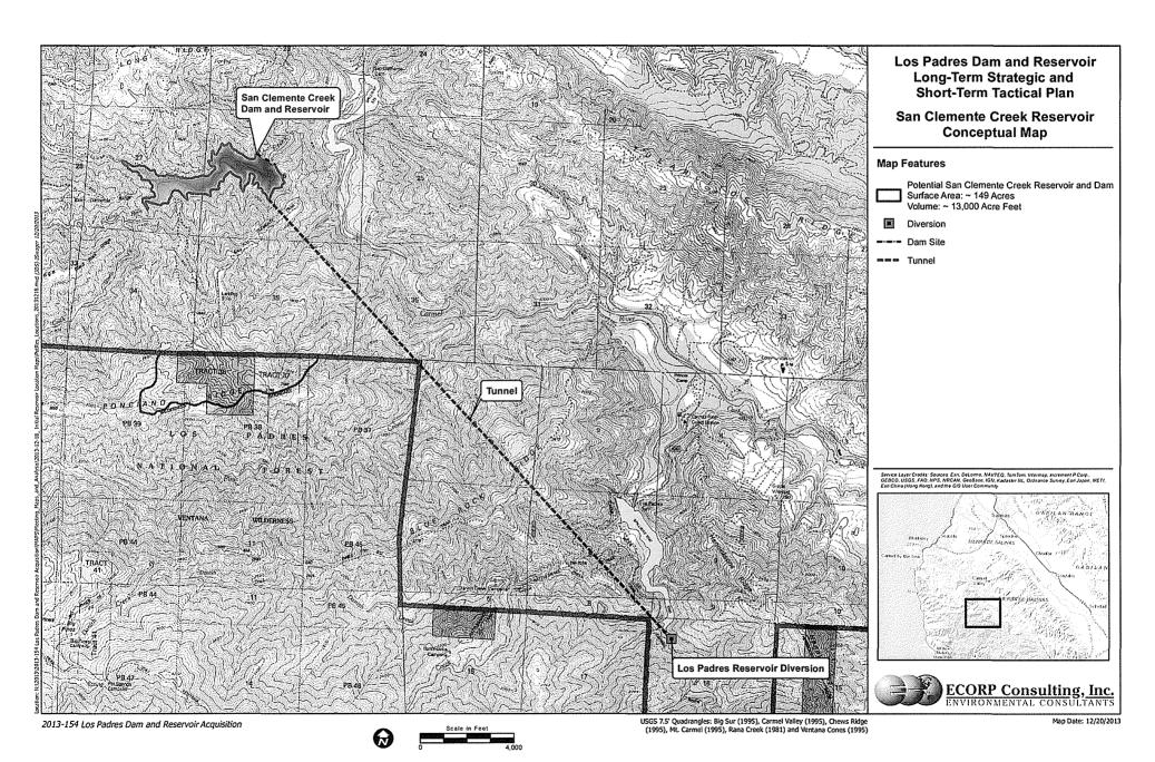
The diversion on the Carmel River (Carmel River Camp Diversion) is located to allow water to flow by gravity into San Clemente Creek Reservoir while locating the diversion as low as possible in the watershed to minimize tunnel length. The San Clemente Creek Dam height was selected to maximize the available storage capacity while allowing runoff from the Carmel River Camp Diversion to flow by gravity to the San Clemente Creek Reservoir.
