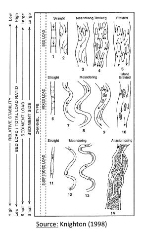
Figure 4-21 Channel pattern characteristics
